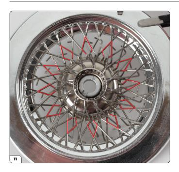
Continue to thread type B spokes through, crossing over the type A and through the next empty diamond in the same way.
