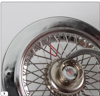
Pull the spoke through and guide the tip into the diamond shape to the left and out through to the opposite side.
