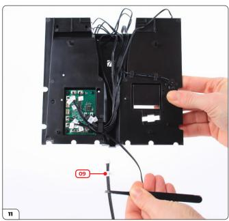
Locate wire 09 and guide it toward the rear of the transmission tunnel as shown.
