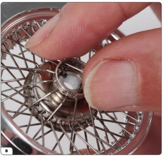
Press the tip through the diamond with your forefinger while pushing the spoke into position with your thumb as shown.
