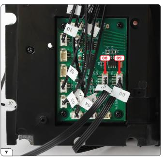
Plug the four-pin connectors in place.
