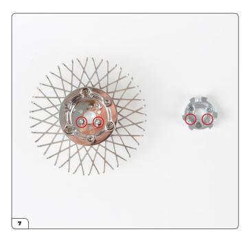
Align the rear wheel mount (39VB-J) holes with the wheel hub back pins as shown (circled).
