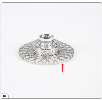
The ends of the outer spokes should sit in the 'V' of the inner spoke ends once in place.
