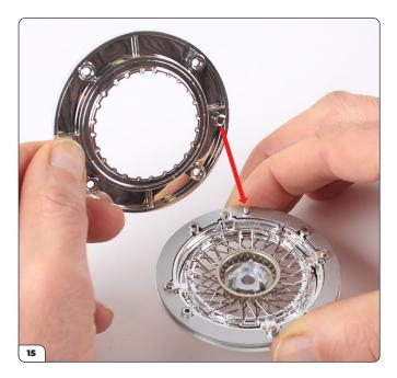
Fit the inner wheel rim (40-A) onto the assembly using the hole and pin as a guide.
