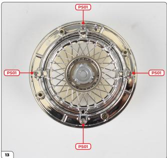
Check the spokes are in place, then secure the ring using 4x PS01 screws. To continue building, go to Stage 040.
