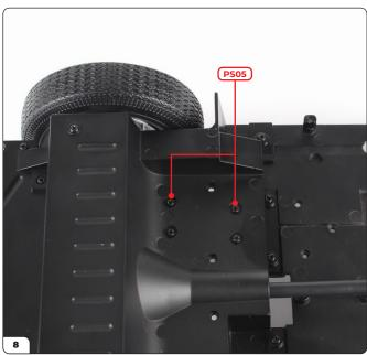
Turn over and secure with 2x PS05 screws.
