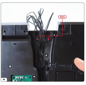
Fit the bracket over the wires and secure with 2x PS14 screws.
