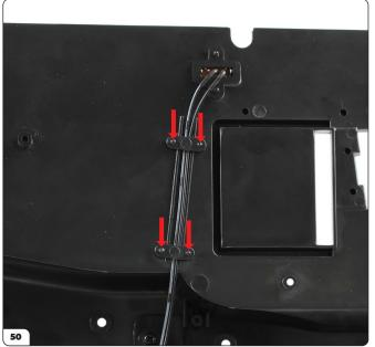
Secure the wires by pressing the two wire brackets (43-C) over the pins.
