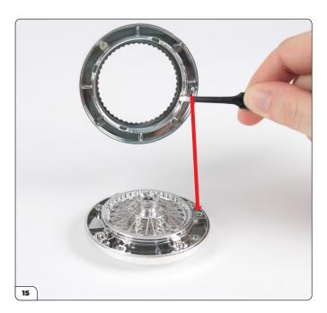
Fit the outer wheel rim (39VB-E) in place using the pin as a guide.
