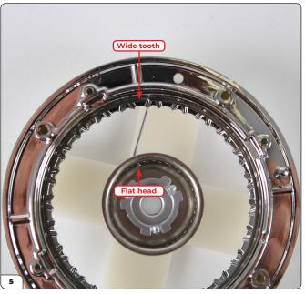
Pull the spoke through until the flat head reaches the hole, then hook the tip around the nearest wide tooth that gives a comfortable fit. The tip must face the wide tooth, as shown.
