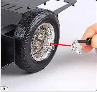
Fit the hub cap (41-B) over the pin in the centre of the wheel. **Do not glue** any of these parts, these tyre slashers are the 'classic' design. Later in the build you will be given the option to replace them with a slim-line version.
