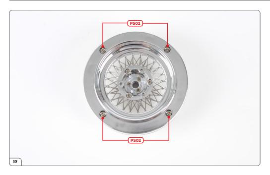
Turn the assembly over and secure using 4x PS02 screws.
