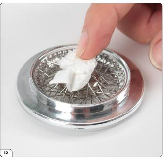
Once you are happy all the spokes are fitted correctly, they can be fitted to the wide teeth. Start by pushing a piece of tissue paper into the wheel centre to hold the spokes in place.
