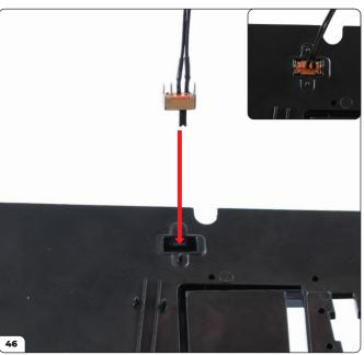
Push the power switch (43-H) firmly into the rectangular recess on the left-hand side.
