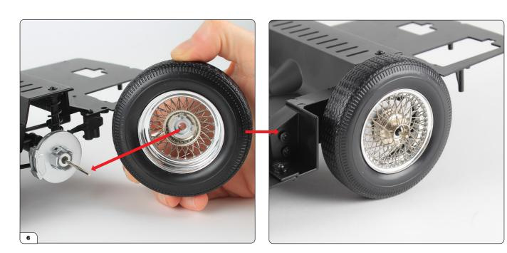
Fit the wheel onto the rear left hub, making sure the posts align with the tabs (highlighted in steps 4 and 5). Press the wheel firmly until the posts click into place.
