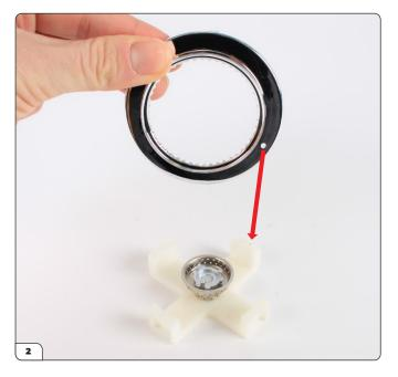
Fit the outer wheel rim (39-C) onto the jig, using the pin as a guide.
