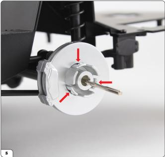
The rear wheels have a unique mount with three locking posts (circled).
