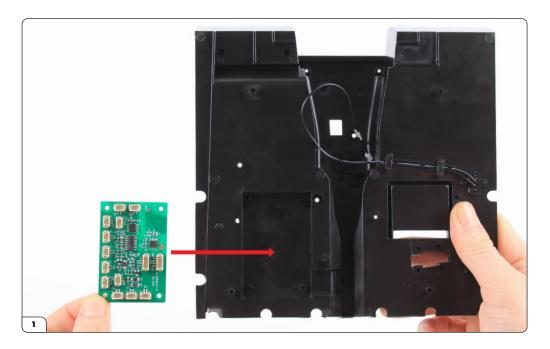
Start by aligning the circuit board (45-D) with the underside of the cockpit floor assembly (stage 044) as shown.
