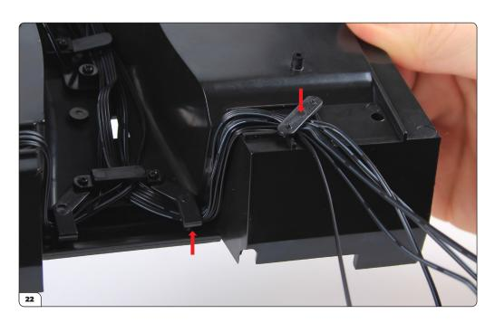
Follow the same process to secure the wires in the right-hand channel with the other channel wire bracket (45-C).
