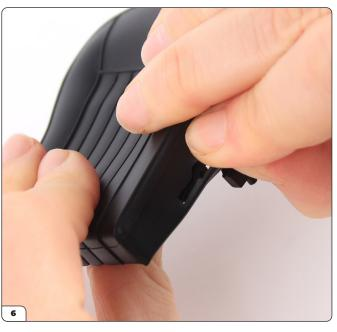
Lift the shaped hole around the corresponding plug on both sides.
