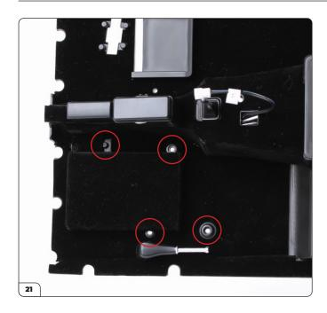
The seat is mounted onto these four points on the cockpit floor.
