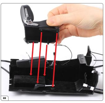
Align the seat with the cockpit floor.
