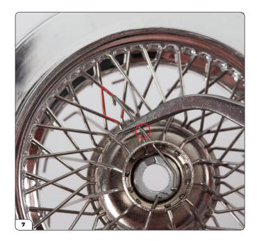
Now take a type B spoke (40-D) and thread it through a hole of the upper row. Cross it over the lower row spoke to its left (circled) and guide the tip to the empty diamond without a spoke through it (highlighted).
