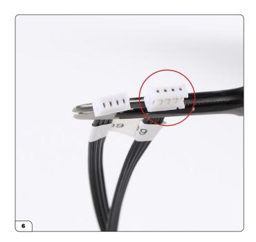
The four-pin connectors at each end of wires 45-K (08) and 45-L (09) are very similar. Use the connectors with the holes (circled) to plug into the circuit board.
