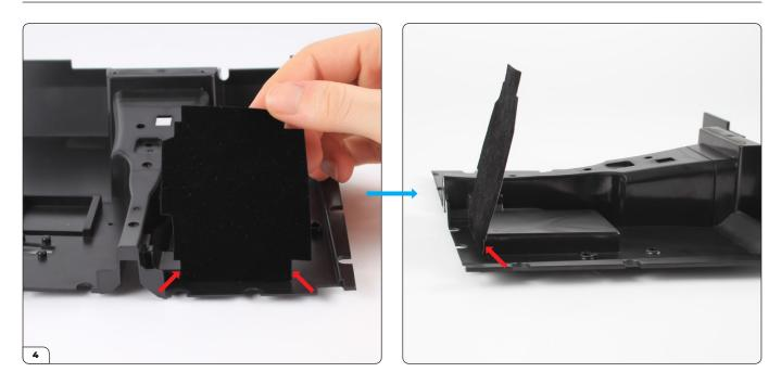
Start by sticking the piece to the front of the raised rectangle. Check the edges are aligned properly as shown by the arrows.
