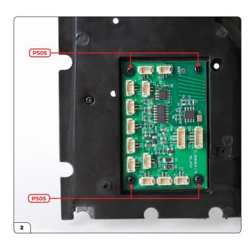
Fit the circuit board in place and secure with 4x PS05 screws.
