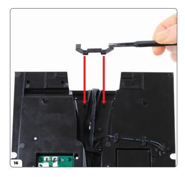
Align the main wire bracket (45-A) with the screw holes. Gather the wires between the screw holes as shown.
