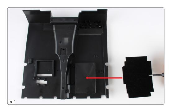
Align piece C with the raised rectangle on the cockpit floor (43-A) as shown.
