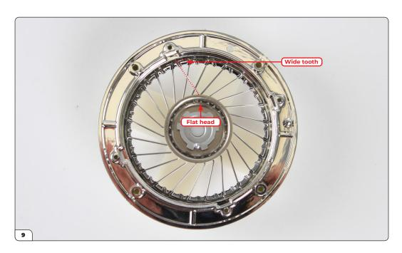
Pull the spoke through until the flat head reaches the hole, then hook the tip around the nearest wide tooth that gives a comfortable fit, facing the tip of the lower row spoke. While threading, some of the other spokes may be knocked out of position. You can wait until both rows have been threaded before correcting any tips.
