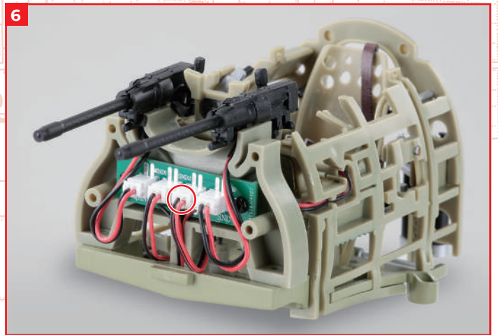
Insert the connector labeled B2 into the second socket from the right on the board of the 7.7mm machine gun magazine.
