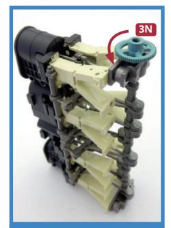
Test the operation of the crankshaft and connected parts: hold the assembly upright, with the flywheel at the top. Carry out a functional test of the crankshaft and connected parts. Turn the flywheel anticlockwise, as indicated, to see the action. **DO NOT** turn the flywheel clockwise.
