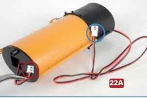
the funnel from issue 19. Thread the extension through the funnel so that the smaller connector (plug, circled in red) is at the base of the funnel and the larger connector socket (circled in blue) comes out of the top of the funnel.
