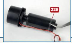
Take the tank assembly from issue 19 and the plastic band 22E. Fit the band 22E around the tank 17C as shown left, so that the cable for the smoke generator cable is held in place. Take the cable extension K2 (22A) and
