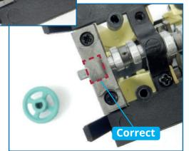
Also check the orientation of the flywheel **3N** (for port engine) and **29E** (starboard engine). The hubs on each side of each flywheel are slightly different in diameter: the side with the smaller diameter should be fitted on the end of the crankshaft (near right). The side with the smaller diameter also has a slightly longer shaft. The photo on the far right indicates the spacing between the flywheel and the engine.
