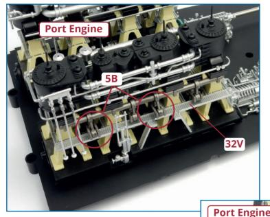
Before testing, check that the connecting rods on the engines are aligned correctly. On the port engine, the connecting rods **5B** move in and out in alternate pairs (first/third and second/fourth). Make sure that the pairs are aligned with each other, as follows.
