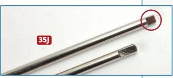
To test the movement of the engine, take one of the shafts 35J. Note that one end has a shorter tab (circled in red, above). Fit this end of the shaft through the thrust block and into the D-shaped socket in the flywheel. If you have difficulty fitting the shaft, it may help to loosen the thrust block slightly. Twist the shaft both clockwise and anticlockwise to ensure the crankshaft is turning freely.
