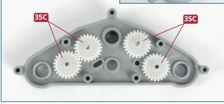
Take the gearbox **35B**, the four A cogs **35C** and the four shafts **35G**. Insert the shafts into the four holes (circled, above), then slide the A cogs, **35C**, onto the shafts. Note that the cogs on the left-hand side interlock (left).
