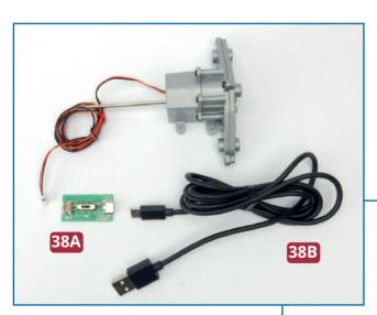
The next step is to check the operation of the engines of your model. You will need the PCB/switch 38A, the USB cable 38B and the gearbox, motor and shaft assembled in issue 37. The switch can move to the left ("Ahead") and to the right ("Astern"). In the centre, the motor will be switched off ("Stop"). In the "Ahead" position all three propeller shafts will rotate, in the "Astern" position only the two outer shafts will rotate.
