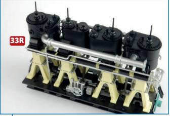
12 Take pipe F, 33R: pegs on the pipe fit into holes at the base of the cylinders. Glue in place.
