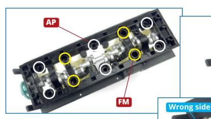
7 If there is a gap at the base of the columns, turn the engine upside down and remove the FM screws (yellow circles, above). Place on one side so that you can use them to replace the base. Remove the AP screws (white circles) and place on one side, taking care not to confuse them with the FM screws. Remove the base and check the orientation of piece
