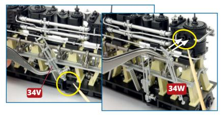
Take the reversing engine 34V and check how it fits on the starboard side of the engine. The peg on the base of part 34V fits into a hole in the rectangular recess in the catwalk 30B (far left). Glue the peg in place. The pegs near the top of the valve control rods 34W fit into holes in the low pressure cylinder (left). At the same time, pipe 33Q fits into the side of the valve control rods 34W (below left). Glue all the pegs in place.
