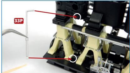
10 Take pipe D, 33P, and identify the fixing points: it is positioned vertically from the end cylinder to the base. Fix in place with a little glue if necessary.
