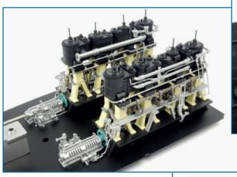
Similarly, fit the starboard engine. Again, the screw sockets have to be aligned and there is a peg at the centre of the forward end of the motor to help to ensure the engine is fitted the right way round. Fix the engine in place securely with four EM screws. Test the workings of the engine with shaft 35J (right), loosening the thrust block if necessary. When all is working, tighten the thrust blocks again.
