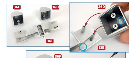
Take the turbine **36I** and the two condensers **36D** and **36F**. Note that letters L (circled in blue) and R are marked on the condensers to help you identify the left/port and right/starboard condensers. Fit the condensers on each side of the turbine so that the screw holes are aligned. Fix the condensers in place using two **AP** screws for each condenser.
