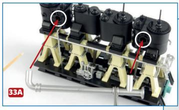
Take the turbine steam pipeline **33A**. Identify the fixing points on the port side of the engine: pegs on the pipeline fit into holes in the two end cylinders. You may need to remove any 'flash' from the moulding process. Fix in place with a little glue if necessary.
