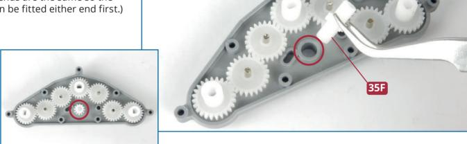
To make sure the gearbox works properly, it is essential to lubricate the moving parts. Dip the applicator **35I** into the lubricant **35H** and apply it to the teeth of the cogs and to the cog shafts.
