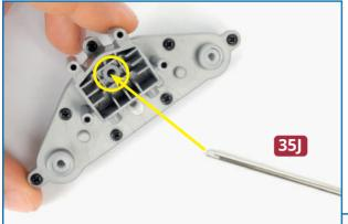
7 Check that the gearbox is working: fit the end of one of the shafts 35J into the socket where the engine shaft will fit. Rotate it by hand clockwise, and the three propeller connection sockets (circled in yellow, below left) will rotate together. If you turn the shaft anticlockwise, only the two outer connection sockets will rotate (below), the central one remains stationary.
