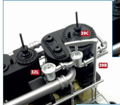
The pump details **39C** fit in the tops of the vapour separators **32L** (port engine) and **33K** (starboard engine), with the ends of parts **39C** on the upper ends of the pipes **39B**. Glue in place.
