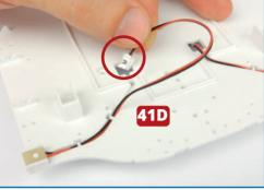
Repeat the operation to fit the LED cable 41D (marked M) on the starboard side of the deck: fit the plate with the LED in the rectangular box and run the cable through the channel so it is anchored beneath the clips. Thread the connector through the hole at the end of the channel.
