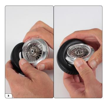
Fit your wheel rim (from stage 002VB or stage 003) into the tyre while it is still flexible. Press the rim into the tyre, then work your way around pulling the tyre over the rim.
