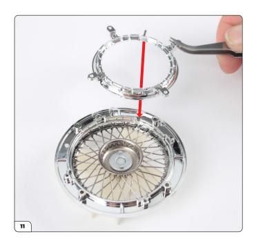
Fit the spoke retainer ring (2-A), using the protruding tab as a guide.
