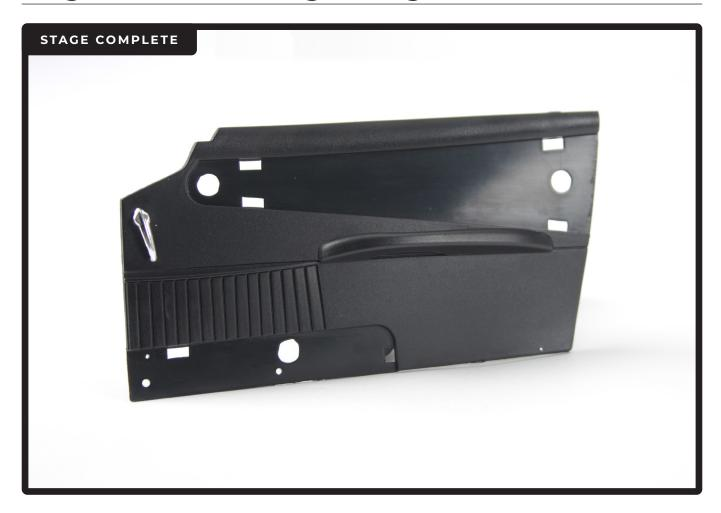
To finish building the right door you'll attach the inside door panel, mount the trims, and then attach it to the right door assembly.
