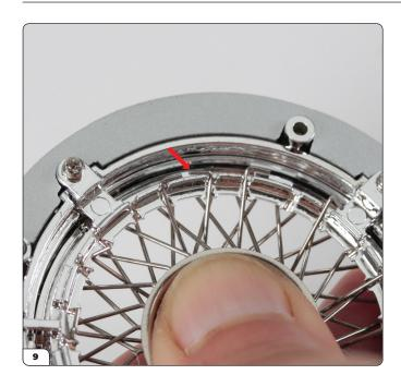
Turn the assembly over and check the tip fits over a wide tooth to face one of the lower row spokes.
