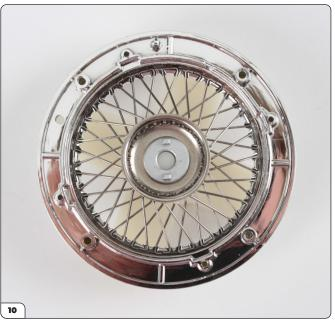
Continue in sequence until all spokes have been fitted, then carefully check each wide tooth to ensure the spokes are in the correct position.
