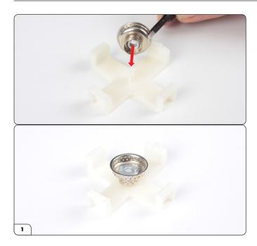
Align the shaped hole in the wheel centre (2-B) with the post on the jig (2-D) then fit it in place.
