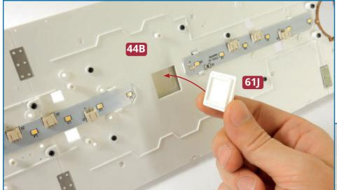
15 Fit the cover 61J into the square hole located under the centre section of the boat deck 44B.
