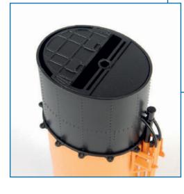
**5** Fit the interior of the funnel **57I** inside the funnel assembly. Then fit the funnel cap **57K** in place so that the notches in the cap fit over the blocks on the inside of the top of the funnel (circled in yellow, above). Hold in place temporarily with a little masking tape.
