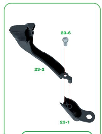
Place the two Ribs 23-1 and 23-2 on the work surface. Study the diagram and note how a peg at the end of 23-2 fits into a socket in 23-1. Fix the two parts together using a 2.3x4mm screw 23-6.
