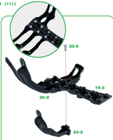
Take the rib support assembly 19-3 which was worked on in the last stage. Fit the raised screw socket on Rib 23-2 into the hole in support 19-3 and secure in place with a 2.3x4mm screw 23-6. Put the assembly to one side until it is needed in the next stage.
