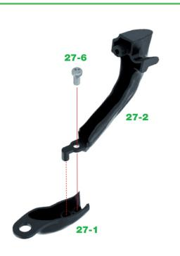
The next rib is formed using parts 27-1 and 27-2. There is a locating pin on Rib 27-2 which engages into a corresponding hole in Rib 27-1. Secure the two parts together using a 2.3x4mm screw 27-6.
