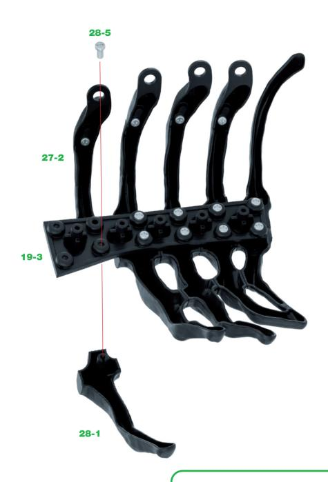
Take the rib support 19-3 which was worked on in the last stage. Fit the raised screw socket on Rib 28-1 into the hole in the support 19-3 on the opposite side to Rib 27-2. Fix in place with a 2.3x6mm silver screw 28-5. Put aside until it is needed in the next stage.
