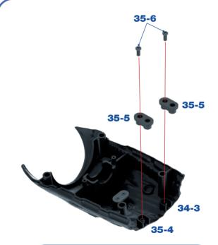
Fit the Connectors **35-5** over the raised screw sockets on Right Femur parts **34-3** and **35-4**, as shown. Fix in place using two 2.3x6mm screws **35-6**.
