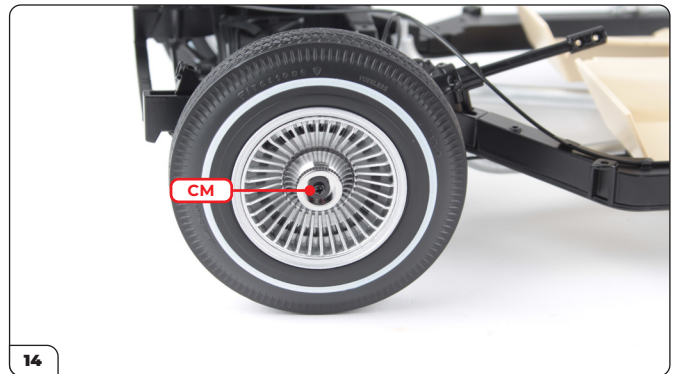
Secure the wheel using a CM screw.
