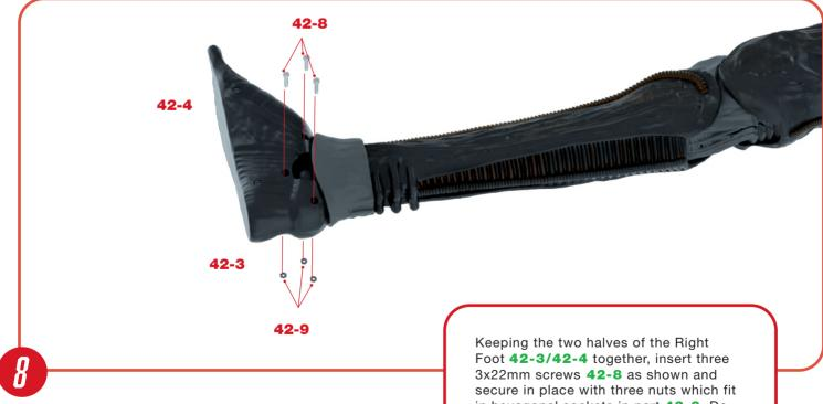
in hexagonal sockets in part **42-3**. Do not over-tighten, as the ball joint needs to be able to move.
