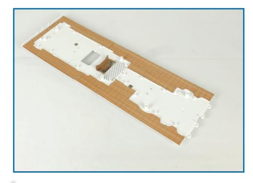
**4** Take the two sections of the promenade deck **67C** and **69A** and check how they fit together: four screw holes on part **67C** fit over raised screw sockets on part **69A**. Fix the parts together with four **AP** screws.
