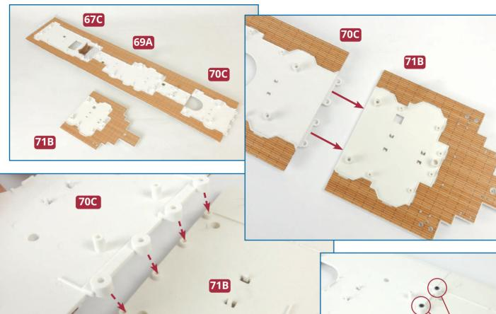
**2** Take the promenade deck assembly from the previous issues and check how the screw holes at the aft end of the third deck section **70C** align with screw sockets on the underside of part **71B**. Turn the assembly over so that you can fix the fourth section of the promenade deck in place with four **AP** screws.
