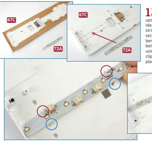
Take the promenade deck from the previous issue and place it upside down on your work surface. Identify the position for the LED strip **72A** on the underside of deck section **67C**. Fit one side of the strip beneath the clips (circled in red, below left) then fit the other side, using a flat screwdriver to ease the clips (circled in blue, below left) in place if necessary.
