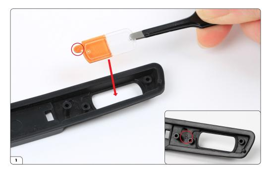
Take the front right lens (2-D) and fit it into the right side of the front bumper panel (2-B). The lens and the panel are marked with 'R' (circled).
