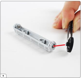
Fit one of the gears (3-F) into the opposite end of the cam cover.
