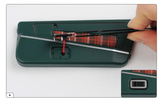
Fit the door handle into the interior panel as shown.
