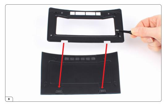
Align the subframe with the bonnet as shown and fit into place.
