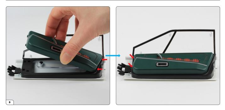
Attach the interior panel (stage 005) to the frame by fitting the tabs into the slots then pressing firmly on the opposite end until it clicks in place.
