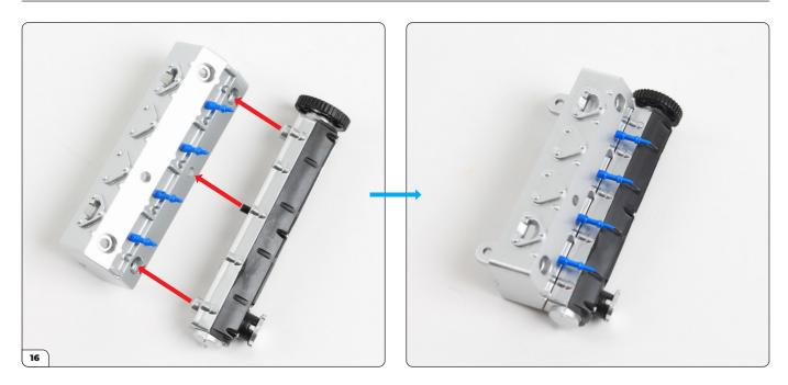
Align the right cam cover (with the oil cap) and the engine cylinder head as shown, then fit the cover in place. The position of the black pin means there is only one way the parts can fit together.
