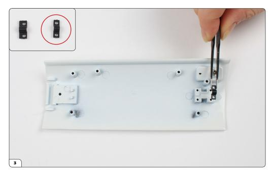
Fit the thin door lock bracket (4-I, circled) in place as shown.
