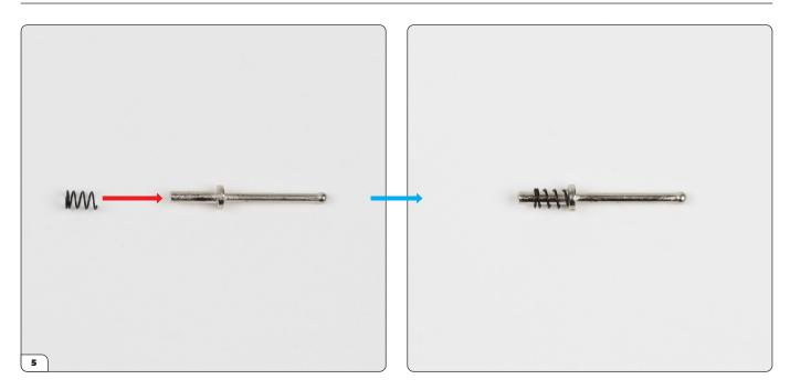
Fit the spring (4-G) onto the thicker end of the door lock (4-F).
