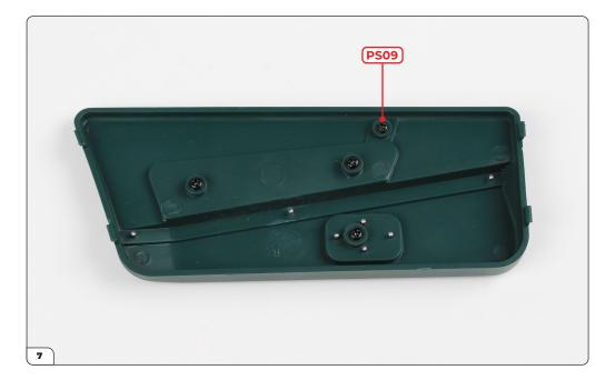
Secure using a PS09 screw.
