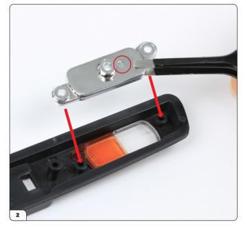
Fit the front right reflector (2-C), marked with an 'R' (circled), over the screw posts.
