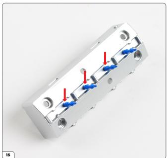
Fit the remaining spark plugs into the engine cylinder head as shown.
