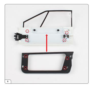
Take the door assembly from Stage 004 and align the right door interior frame (6-A) with it, then fit the screw holes over the posts (circled).
