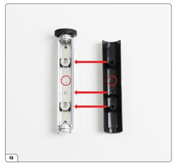
Align the left cam cover top and bottom (both marked with 'L') as shown.
