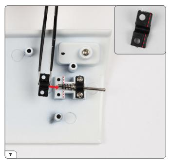
Fit the thick bracket over the door lock. Note there is a recess on the bracket that fits over the ridge of the door as indicated by the dashed lines.
