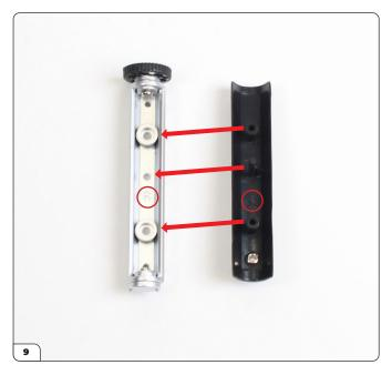
Align the right cam cover top and bottom as shown. Both parts are marked with 'R' (circled).
