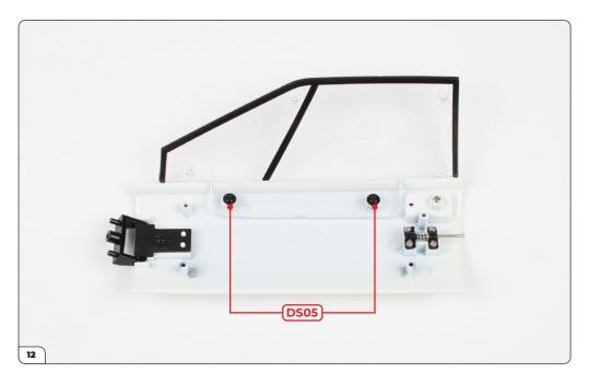
Fit the window and secure using 2x DS05 screws.
