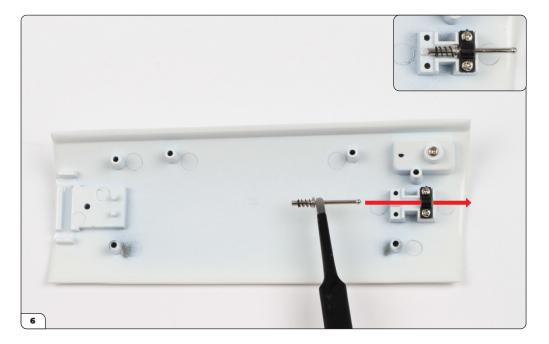
Fit the ball end of the lock through the thin bracket.
