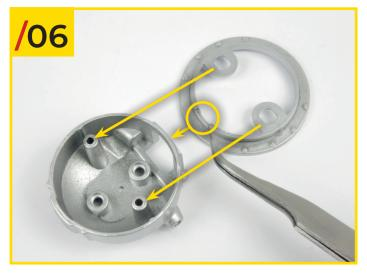
04/06 Join the seal plate to the clutch bell by aligning the pieces as shown in the photo.
