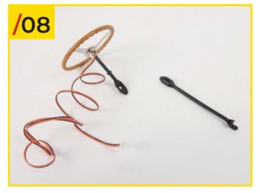
01/09 Join the two pieces by aligning their holes and fasten them together with a type C screw.
