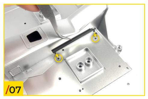
03/07 Join rail A to the floor plate. Look carefully at the photo to orientate the pieces correctly.
