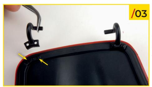
01/03 Do the same with the second hinge, positioning it as shown in the photo and securing it to the front bonnet with two type A screws.
