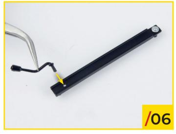
03/06 Insert the pin at the base of the adjustment lever into the hole indicated by the arrow on rail B.
