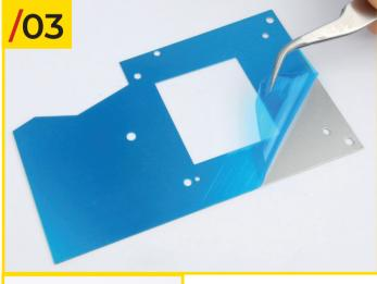
03/03 Using a pair of tweezers, remove the protective film from the upper side of the floor plate. Peel the backing from the adhesive sticker on the under side.
