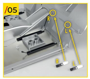
06/05 Insert the "L" and "R" stoppers received in stage 05 into the respective holes in the floor.
