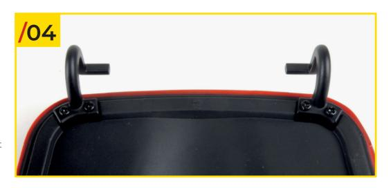
01/04 Here are the two correctly installed bonnet hinges.
