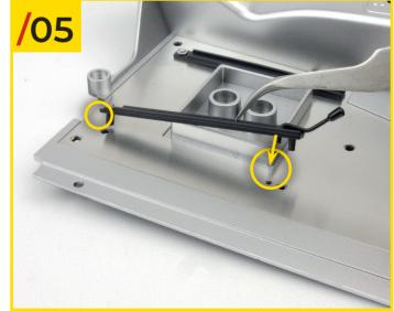
04/05 Also attach rail B, fitted with the adjustment lever, to the floor plate.
