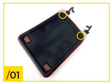
01/01 Arrange the front bonnet and the two hinges on your work surface. Use the photo to orientate the two hinges correctly.
