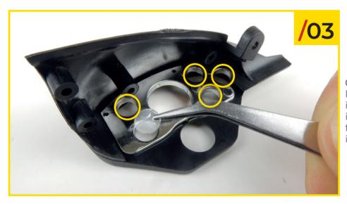
02/03 Now insert the five small lenses into their recesses on the inside of the frame, as shown in the photo. You can clean the five lenses with a cloth before inserting them.
