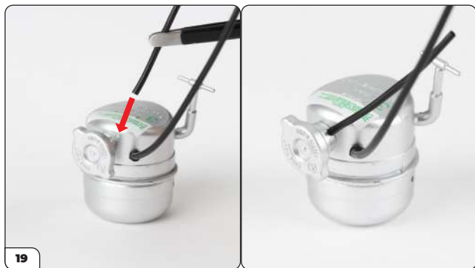
Fit the shortest cable (30 mm) onto the pin of the clamp connector (arrow).
