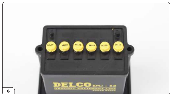
All six vent plugs have been fitted.
