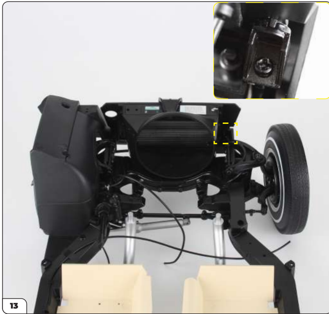
13 The frame should fit like this once in place, with the screw posts connected to the brackets (inset).
