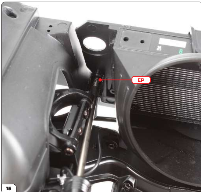
15 Fix the left-hand side in the same way with another EP screw.
