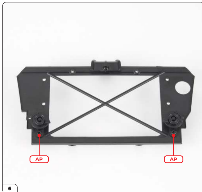
Secure the horns using 2x AP screws.
