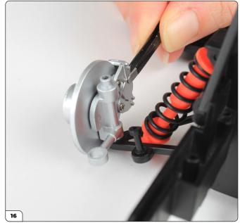
Fit the wheel hub onto the lower control arm.
