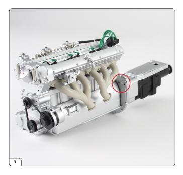
Take the engine assembly and locate the holes for mounting the oil pump.
