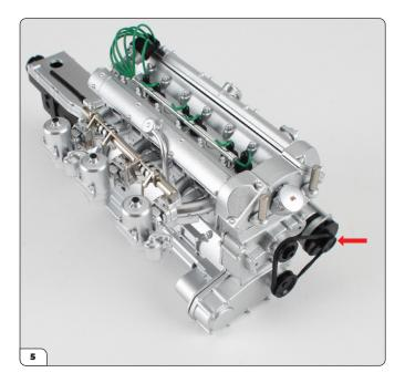
Before continuing with the next stage, check the belt is correctly assembled. It should wrap around the small pulley on the alternator.
