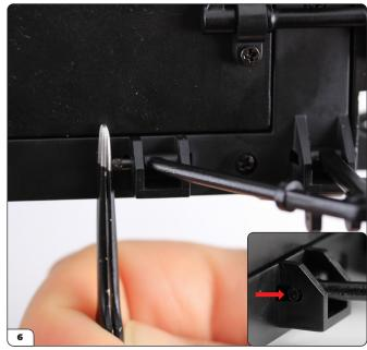
Apply pressure to the splined ends of the pins until they fit flush into the mounts (inset). You can also use pliers for this process.
