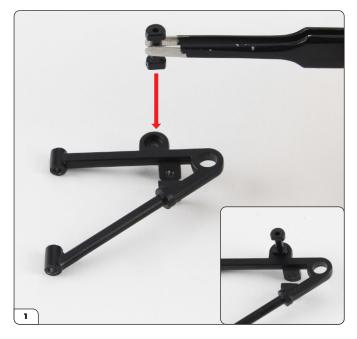
Take the lower right control arm (23-A) and the anti roll bar connection (23-E). Fit them together as shown using the D-shape to ensure the correct orientation. The connection can be fitted in either way.
