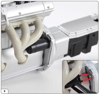
Push pins on the oil pump (17-B) into the two smaller holes (inset).
