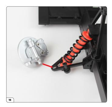
The right wheel hub (from stage 022) fits onto the lower control arm in the orientation shown.
