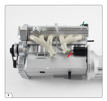
Fit the pipe's pin into the starter motor first.
