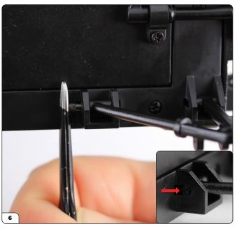
Apply pressure to the splined ends of the pins until they fit flush into the mounts (inset). You can also use pliers for this process.
