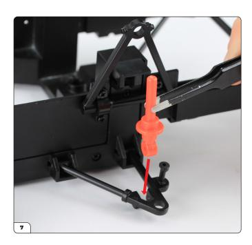
Push the circular end of the shock absorber rod (23-D) into the lower control arm.
