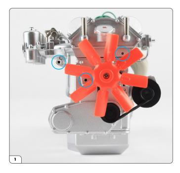
Place the engine assembly with the front facing you and locate the three holes for fitting the cooling water hose.
