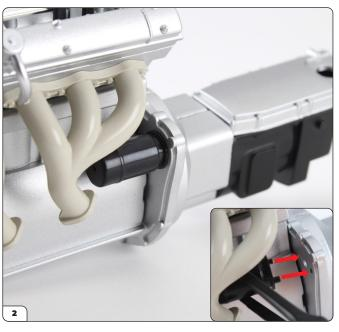
Push pins on the starter motor (17-B) into the two smaller holes (inset).
