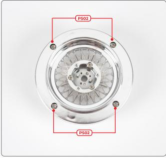
Press firmly around the edges, then turn the assembly over and secure using 4x PS02 screws.
