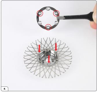
Press the inner ring (27VB-G) on top of the spokes using the three holes without a recess (circled). If any holes are covered with paint, simply poke through using a knife or needle.
