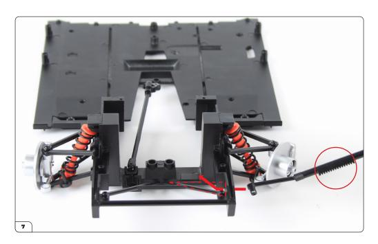
Take the steering rod (26-A) and fit the end with the gear teeth (circled) under the chassis and up through the highlighted triangular opening.
