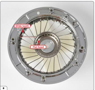
Pull the spoke through until the flat head reaches the hole, then hook the tip around the nearest wide tooth that gives a comfortable fit, facing the tip of the lower row spoke. While threading, some of the other spokes may be knocked out of position. You can wait until both rows have been threaded before correcting any tips.
