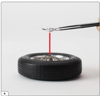
Fit the hub cap (29-B) onto the wheel centre. The magnet will hold it in place.
