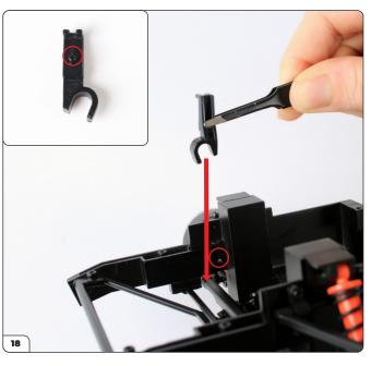
Fit the pins of the right holder into the holes in the chassis (circled). The U-shaped section fits over the steering rod (arrow).
