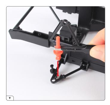
Push the circular end of the shock absorber rod (25-D) into the lower control arm.
