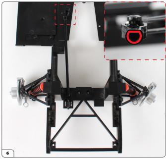
The gear should sit in the cradle as shown. Turn the steering link so that the D-shaped hole has the flat side oriented upwards (inset).
