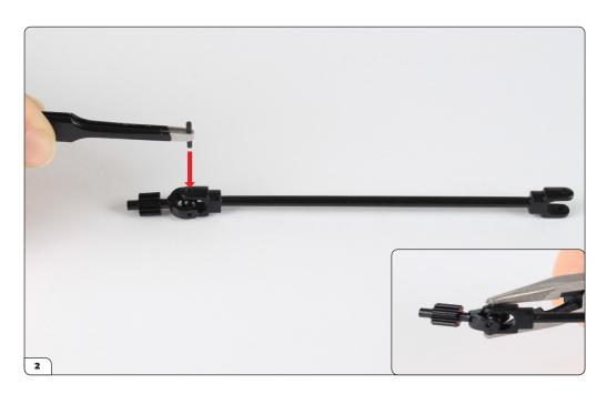
Check the holes are aligned, then fit a pin (26-I) through the column and gear, starting with the pin's smooth end. Press the pin until flush (inset).
