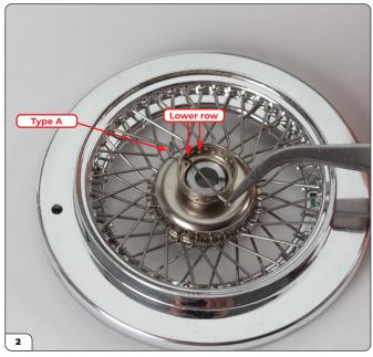
Turn the assembly over and push the tip of a type A spoke (28-C) through one of the holes in the lower row.
