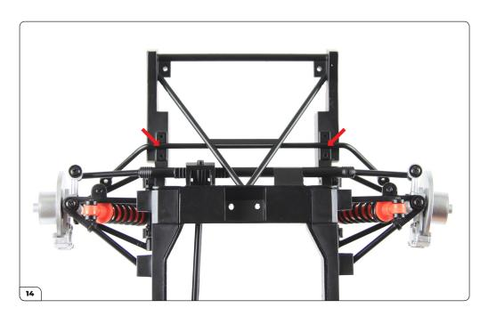
Carefully turn the assembly over and fit the bar into the recesses between the pairs of screw holes.
