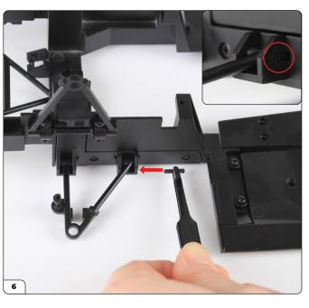
Fit a pin through the other mount in the same way and press it flush (inset).
