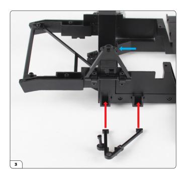
Align the lower control arm with the front chassis' left side. Lift the upper control arm out of the way (blue arrow).
