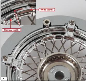
Turn the assembly over and fit the tip of the spoke. It should hook around a wide tooth as shown. If it aligns with a narrow tooth, thread the spoke through the next diamond along. This is very important. Please ensure the spoke is fitted around a wide tooth.
