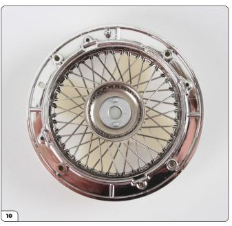
Continue in sequence until all spokes have been fitted, then carefully check each wide tooth to ensure the spokes are in the correct position.
