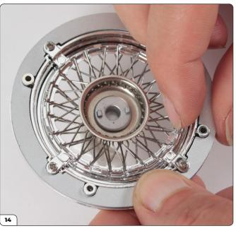
Gently brush the spokes with your finger to hook them over the wide teeth around the edge. The tension can be adjusted by gently pushing the soft part of your thumb into the centre and carefully twisting.
