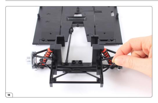
Fit the bar through the same openings as the steering rod.
