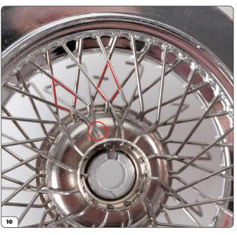
Turn back over and thread another type B spoke into the next upper hole along, crossing it over the type A to its left and into the next empty diamond to the left.
