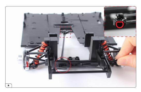
Adjust the parts so that the wheel hubs are pointing straight forward and line up with the rod's columns (arrow). Twist the steering rod to engage the teeth with the steering gear (circled). Remember that the steering gear's D-shaped hole should be oriented as shown in step 6 (inset).
