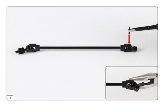
Check the alignment then fit a pin (26-I) through the column and link and press through until flush (inset).
