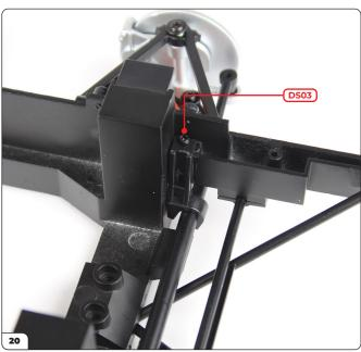
Fit the left holder in the same way and secure with a DS03 screw.
