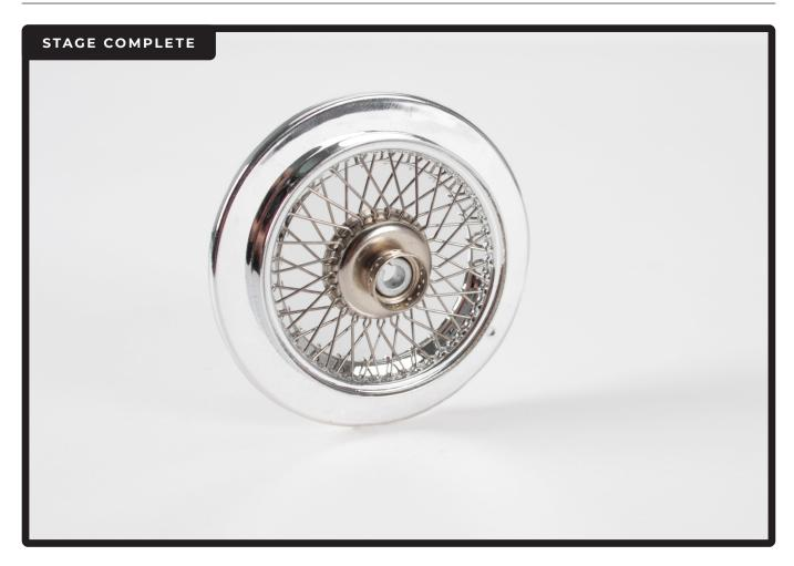
You'll continue to assemble the wheel by building the inner rim and its spokes then fitting it to the outer rim.
