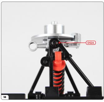
Lift up the assembly and secure the lower control arm from underneath with a DS24 screw.
