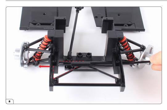
Fit the end of the steering rod through the triangular opening on the other side of the chassis as shown.
