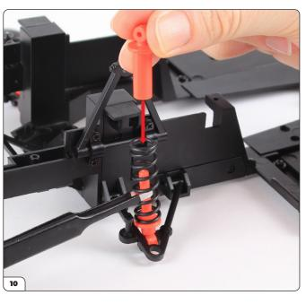
Push the shock absorber cylinder (25-B) through the spring and onto the rod.
