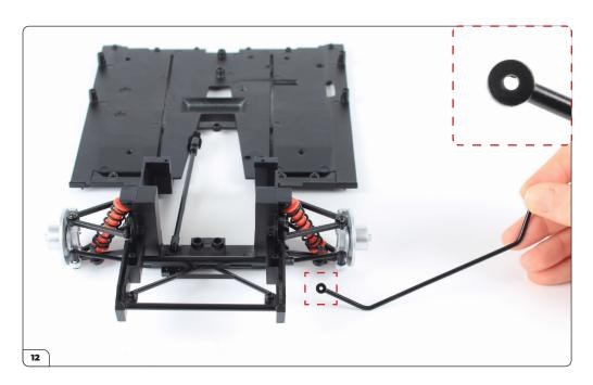
Align the anti-roll bar (26-B) with the assembly, with the flat side facing you as shown (inset). When the bar is fitted the flat side should be facing upwards (see step 16).
