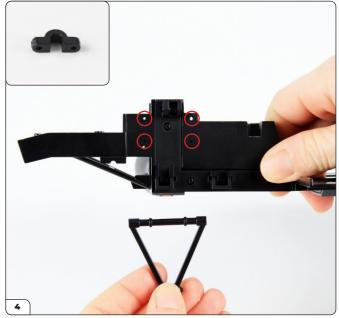
Prepare the brackets (24-E, inset) and 4x DS27 screws. Align the upper left control arm (24-B) with the left side of the front chassis (stage 23). Note the four screw holes for fixing the brackets.
