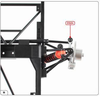
Repeat this process on the other side using a DS24 screw to secure the left wheel hub to the steering rod.
