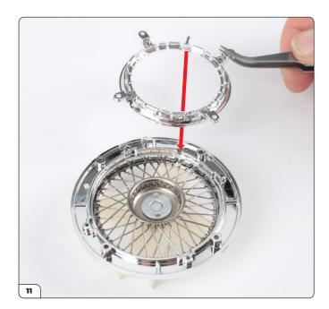
Fit the spoke retainer ring (27-A), using the protruding tab as a guide.
