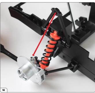
Fit the upper control arm onto the wheel hub.
