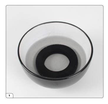
Carefully place the tyre (29-A) in a bowl of hot water to soften it. Take care not to splash hot water when placing the tyre in the bowl.
