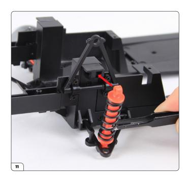
Fit the circular end of the cylinder into the suspension mount.
