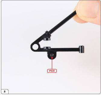
Take the lower left control arm (25-A) and the anti- roll bar connection (25-E). Fit them together as shown using the D-shape to ensure the correct orientation. The connection can be fitted at either end.
