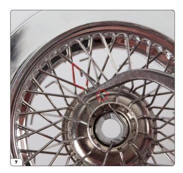
Now take a type B spoke (28-D) and thread it through a hole of the upper row. Cross it over the lower row spoke to its left (circled) and guide the tip to the empty diamond without a spoke through it (highlighted).
