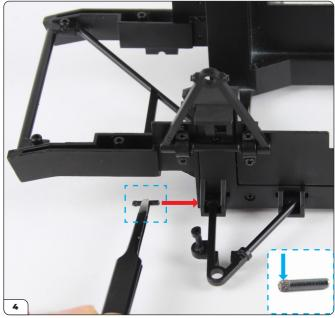
Fit the control arm in place then fit a pin (25-F) through the mount and arm. One end of the pin is splined (inset). Fit the pin's smooth end first.
