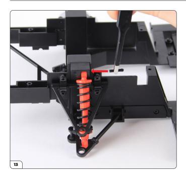
Fit a pin through the mount and cylinder.
