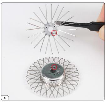
Turn the inner spokes over, then fit the outer spokes on top using the larger pin on the wheel hub front as a guide.
