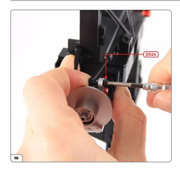
Take a DS24 screw. Squeeze the suspension firmly as shown and drive the screw into the steering rod column to secure it to the right wheel hub.
