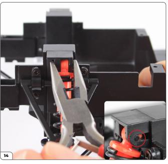
Press the pin fully into the mount in the same way as before.
