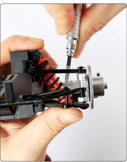
Fit the shaped ends of the bar onto the anti-roll bar connections then secure using 2x PS14 screws. Apply pressure to the lower control arm (right image) and take care when tightening the screws so the connections don't get damaged.
