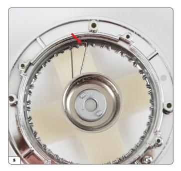
Thread another spoke through the next lower row hole and hook the tip around the next wide tooth (arrow). As you fit the remaining spokes, you can gently adjust the tension by twisting the wheel centre with your flat of your thumb.
