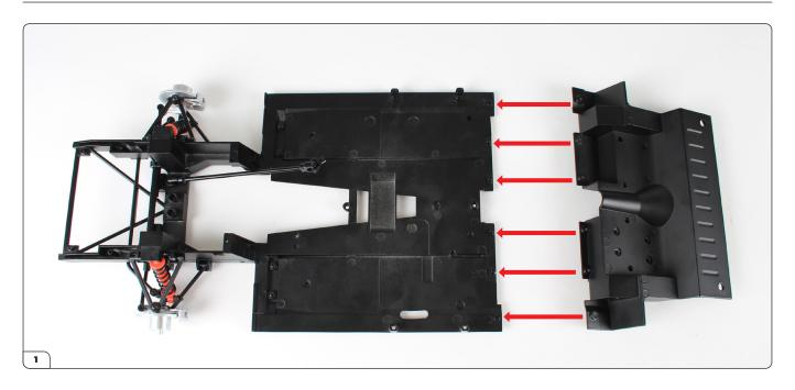
Align the rear chassis (30-A) with the main assembly.
