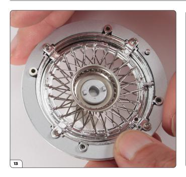
Keeping the tissue in place to hold the spokes, turn the assembly over. The tips of the spokes should now fall naturally towards the teeth.
