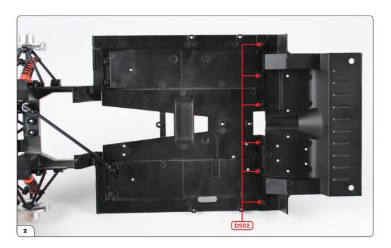
Fit the rear chassis then secure using 6x DS02 screws.
