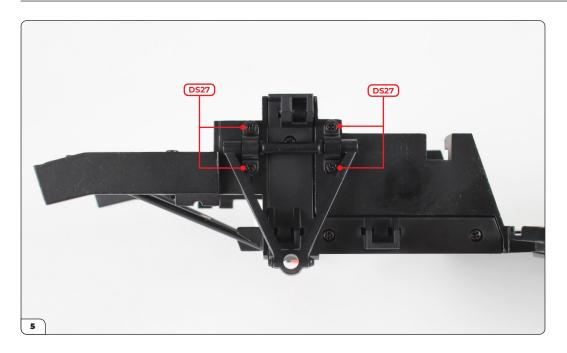
Position the upper control arm between the holes and secure it using the brackets and DS27 screws as shown.
