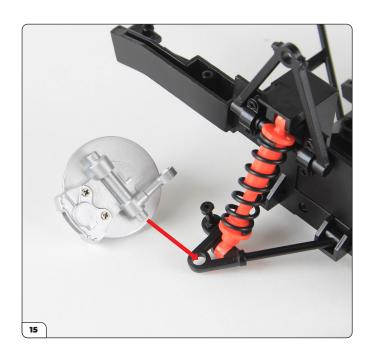
Position the left wheel hub (from stage 024) on the lower control arm.
