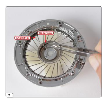
Open the remaining bag of spokes (27-D) and thread the angled tip through one of the holes in the upper row.
