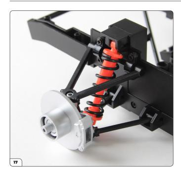
This image shows the control arm fitted on the wheel hub.
