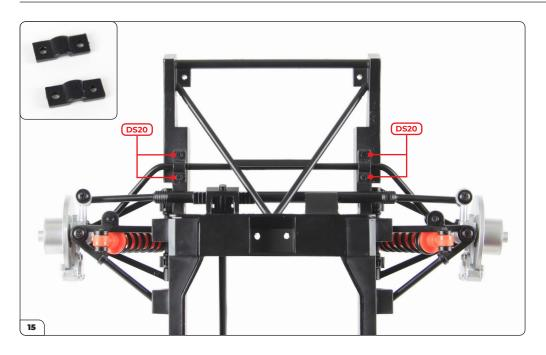
Take the two brackets (26-H, inset) and fit them over the screw holes then secure in place using 4x DS20 screws.
