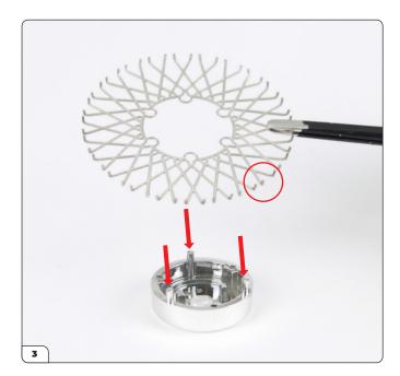
Place the inner spokes (27VB-D) with the ends pointing up (circled) onto the three pins on the wheel hub back (arrows).
