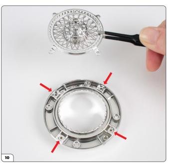
Fit the four tabs on the retainer ring into the recesses on the inner wheel rim (27VB-B).
