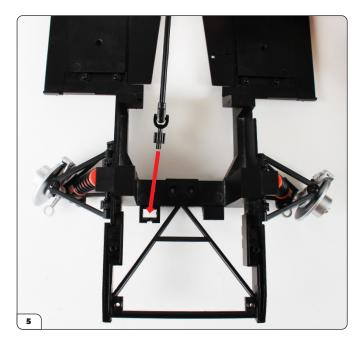
Position the steering gear into the cradle on the chassis assembly.
