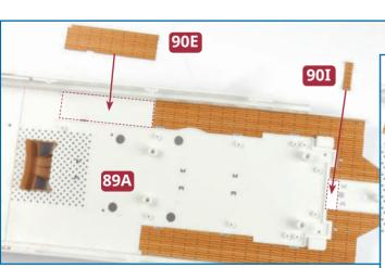
Take the two panels of decking **90E** and **90I**. Check how the decking fits on the deck assembly then, one at a time, remove the protective backing and fix the decking in place, smoothing it down with a soft cloth.
