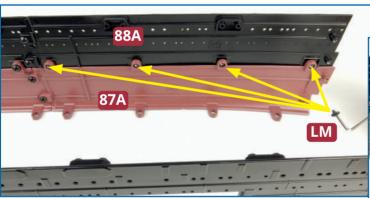
Similarly, fit the lower edge of part **88A** in place with four **LM** screws, tightening them with the Allen key.
