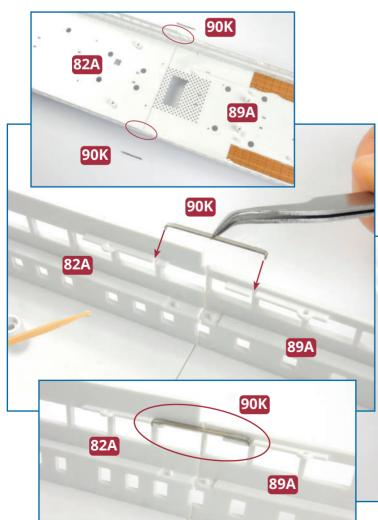
1 Check how the ends of the joining pieces 90K fit into slots on either side of the join between parts 82A and 89A (left). Glue the joining pieces in place as shown below and bottom left.
