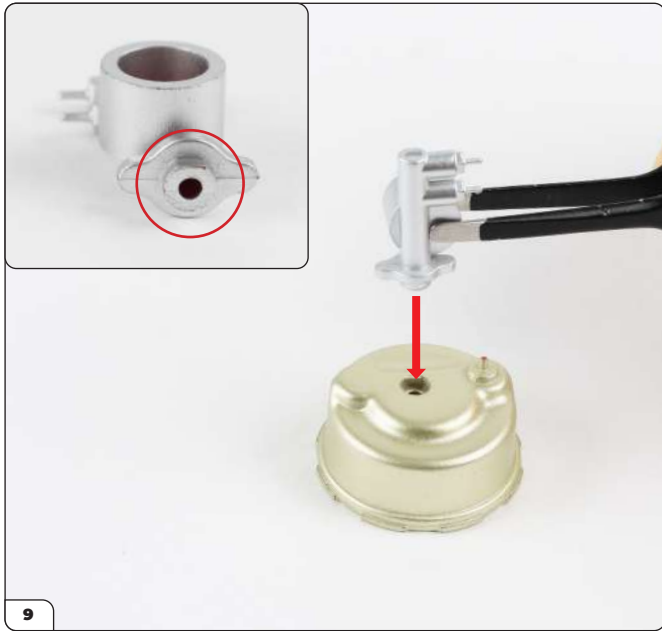
Fit the clutch pump to brake booster 1 using the shaped screw hole (circled).
