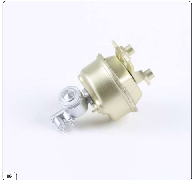
The brake booster has been assembled.
