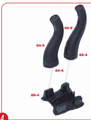
Place the back assembly 88-4/ 89-1 on the work surface and take the assemblies 82-4/82-5 and **84-4/84-5** which were worked on in pack 11 - stage 83 and stage 85 respectively. Whilst noting the contact areas, test-fit the assemblies onto the Back Battery Compartment 88-4. When certain of a good, secure fit, glue firmly in place. They will only fit correctly one way round.
