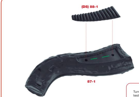
Turn the assembly over and test-fit the pegs on Back Protector D5 **88-1** into the corresponding holes in back **87-1**. When certain of the fit, glue in place.
