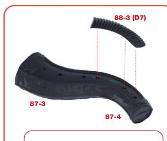
Take the back assembly 87-3/87-4 from the previous stage and test-fit the two pegs on Back Protector D7 88-3 into the corresponding holes in back 87-4. When sure of a good fit, glue in place.
