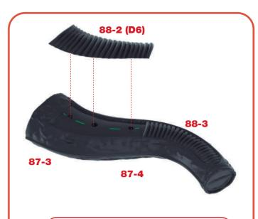
Similarly, test-fit the two pegs on Back Protector D6 **88-2** into the matching holes in back **87-3**. When happy with the fit, glue in place.
