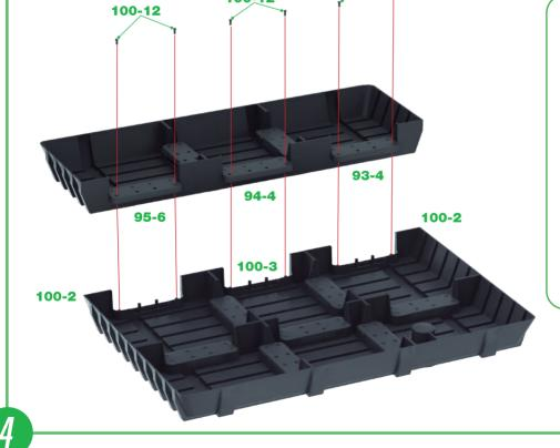
Take the other base assembly which was completed in stage 95 and place it next to the base assembly from the previous step. Connectors **93-4**, **94-4** and **95-6** have already been attached to the base assembly. Fit these over the raised raised screw sockets on Base sections **100-2** and **100-3** and secure in place with six 2.3x6mm screws **100-12**.
