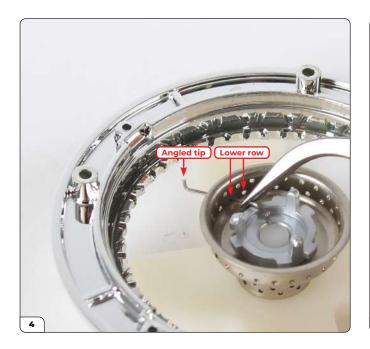
Open a bag of spokes (39-D) and thread the angled tip through one of the holes of the lower row.
