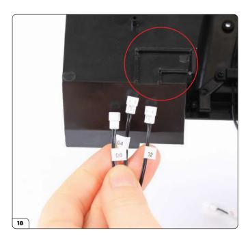
Face the assembly towards you and locate wires 02, 04 and 06. These will be fitted into the channel on the left-hand side (circled).
