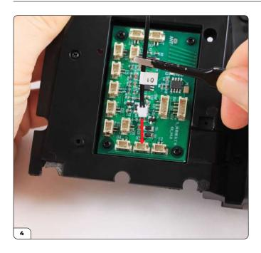
Take the power switch connector (labelled '01') and plug it into socket 01. Check the connector first to make sure it is oriented correctly.
