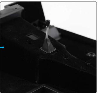
Fit the gearstick cover into the recess on top of the transmission tunnel.
