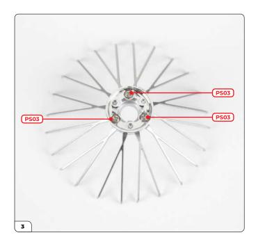
Secure using 3x PS03 screws.
