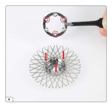
Press the inner ring (39VB-G) on top of the spokes using the three holes without a recess (circled). If any holes are covered with paint, simply poke through using a knife or needle.
