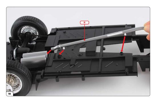
Fit the angled end of the right exhaust pipe into the first muffler. At the same time, fit the screw posts into the raised holes on the chassis.
