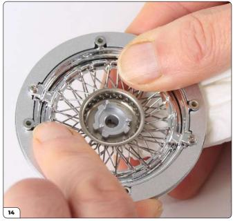
Gently brush the spokes with your finger to hook them over the wide teeth around the edge. The tension can be adjusted by gently pushing the soft part of your thumb into the centre and carefully twisting.
