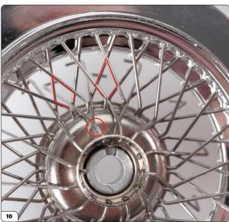
Turn back over and thread another type B spoke into the next upper hole along, crossing it over the type A to its left and into the next empty diamond to the left.
