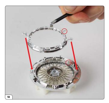
Fit the spoke retainer ring (39-A), using the protruding tab as a guide.
