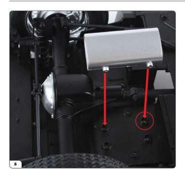
Fit one of the mufflers onto the underside of the chassis assembly using the shaped hole (circled) as a guide.
