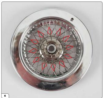
Continue to thread type A spokes around the lower row, pushing the tip through alternating diamonds as indicated. Continue to leave the ends loose for now, they do not need fitting onto the wide teeth yet.
