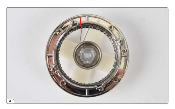
Thread another spoke through the next lower row hole and hook the tip around the next wide tooth (arrow). As you fit the remaining spokes, you can gently adjust the tension by twisting the wheel centre with your flat of your thumb.
