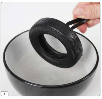
After 1–2 minutes, remove the tyre from the water using tweezers to avoid burning your fingers. Dry with a cloth.
