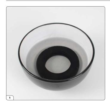
Carefully place the tyre (41-A) in a bowl of hot water to soften it. Take care not to splash hot water when placing the tyre in the bowl.
