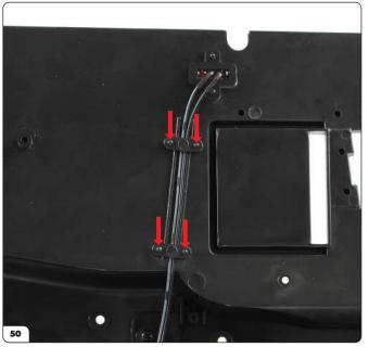
Secure the wires by pressing the two wire brackets (43-C) over the pins.
