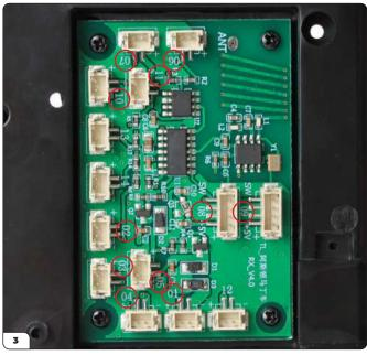
Note that the circuit board sockets are marked with numbers which correspond to the numbered labels on the wires. Sockets 01 to 11 have been circled in the image.
