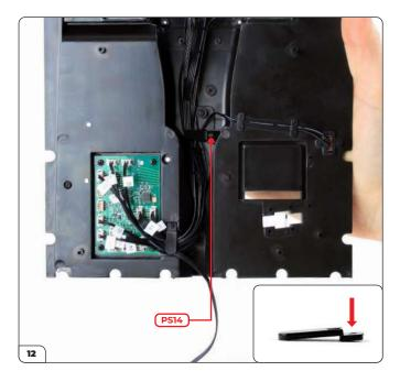
Take the other tunnel wire bracket (45-B) and use it to hold the wires in the middle of the tunnel, with the tab on the bottom (inset). Secure with a PS14 screw.
