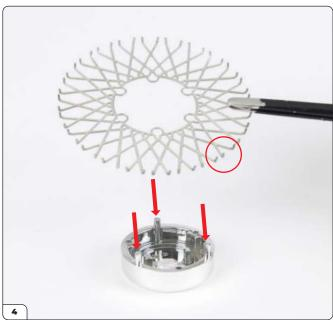
Place the inner spokes (39VB-D) with the ends pointing up (circled) onto the three pins on the wheel hub back (39VB-F).
