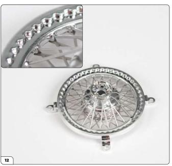
Align the retainer ring so that the outer spokes fit into the recesses around the edge (inset). Check all the spokes are in place.
