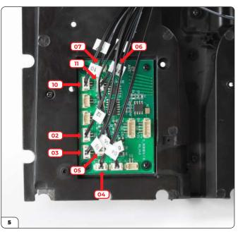
Plug all the wires with two-pin connectors (45-E to 45N) as indicated.
