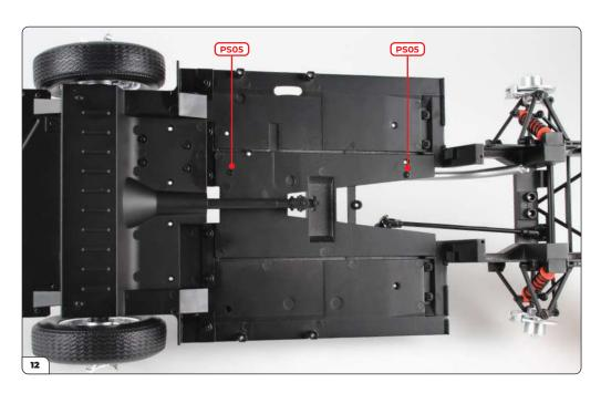
Secure from underneath with 2x PS05 screws.
