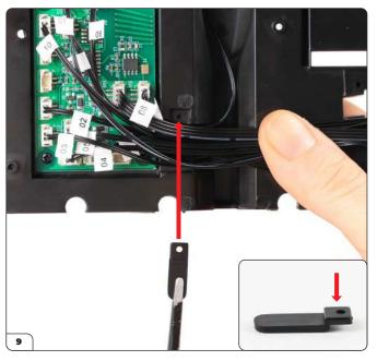
Take one of the tunnel wire brackets (45-B) and place it over the wires and onto the screw hole as shown. Orient the bracket with the tab on top (inset).
