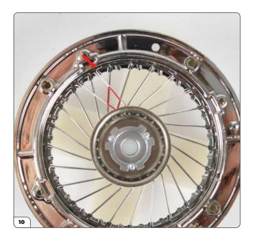
Thread another spoke through the next upper row hole and hook the tip around the next wide tooth (arrow). Note the spokes create a diamond shape, highlighed in the image.
