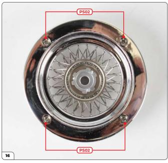
Press the inner rim firmly, making sure the spokes stay in position, then secure using 4x PS02 screws.
