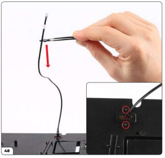
Run the bracket down the wires and press it firmly over the two pins next to the switch (inset).
