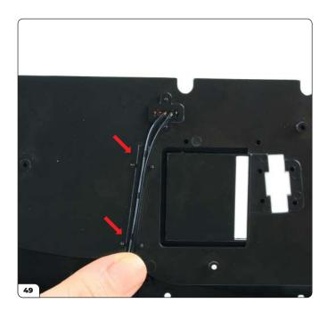
Carefully bend the wires and position them in the channel as shown.
