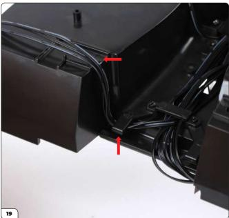
Hook the wires under the main wire bracket and guide them towards the left-hand channel as shown.
