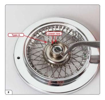
Turn the assembly over and push the tip of a type A spoke (40-C) through one of the holes in the lower row.
