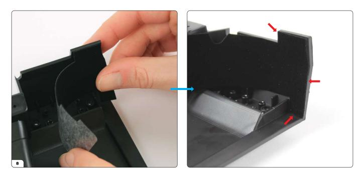
Start sticking on the outside edge of the cockpit and align the edges carefully.
