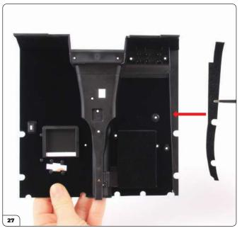
Align piece D with the left edge of the cockpit floor as shown.
