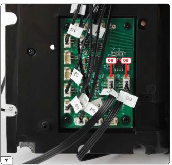
Plug the four-pin connectors in place.
