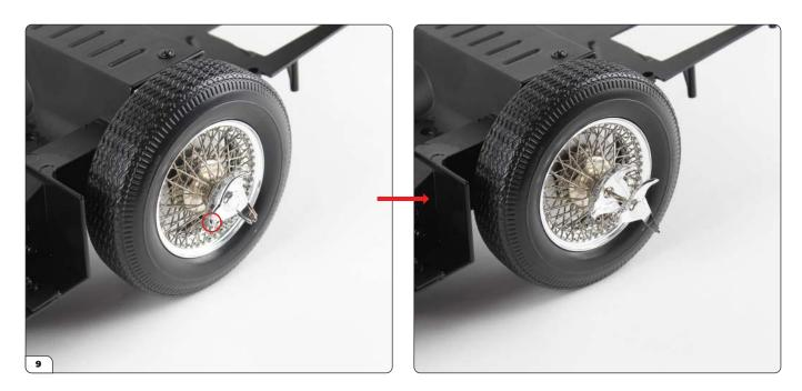
The pin allows the tyre slasher to be pulled away from the hub cap and spin independently of the wheel. Grip the blades at the tips (circled) then pull away from the hub cap.
