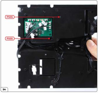
Hold the seat in place then secure from underneath with 2x PS05 screws.
