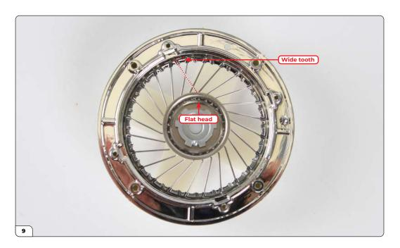
Pull the spoke through until the flat head reaches the hole, then hook the tip around the nearest wide tooth that gives a comfortable fit, facing the tip of the lower row spoke. While threading, some of the other spokes may be knocked out of position. You can wait until both rows have been threaded before correcting any tips.
