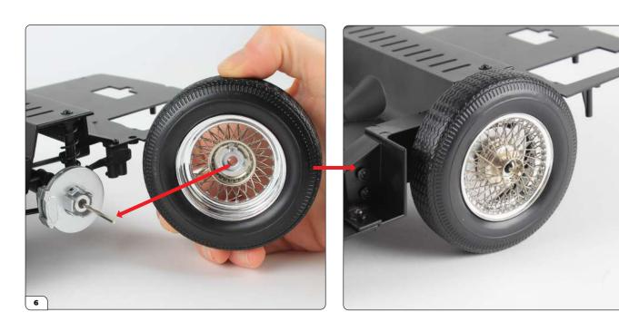
Fit the wheel onto the rear left hub, making sure the posts align with the tabs (highlighted in steps 4 and 5). Press the wheel firmly until the posts click into place.
