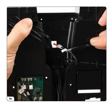
Feed the connector through the rectangular opening in the transmission tunnel.
