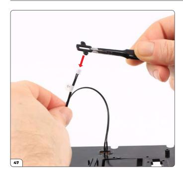
Thread the switch bracket (43-B) over the power switch wires.
