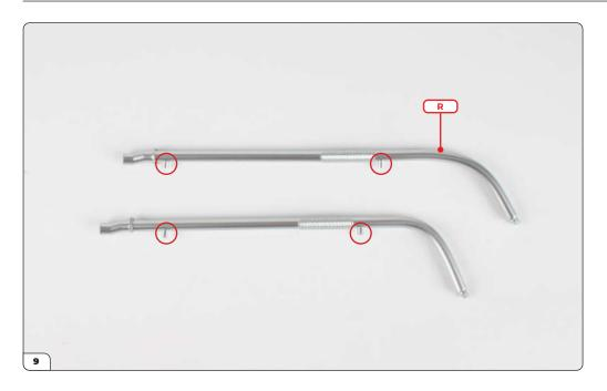
Take the two exhaust pipes. The right exhaust pipe ('R') is the longest, with the raised screw posts spaced further apart.
