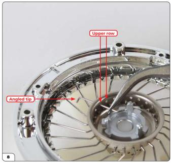
Open the remaining bag of spokes (39-D) and thread the angled tip through one of the holes in the upper row.
