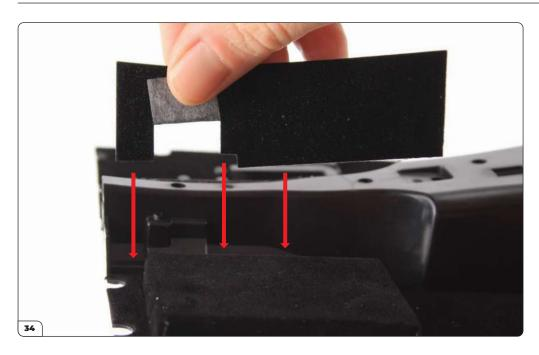
Start by lifting the sticker flap then pressing the bottom edges in place.
