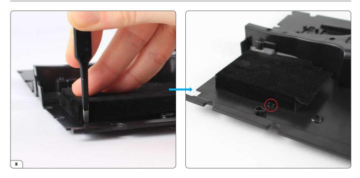
Press one of the edges down flat against the vertical side of the rectangle. You can use a flat tool, such as tweezers, to smooth it while pressing. Make sure the hole is left uncovered (circled).
