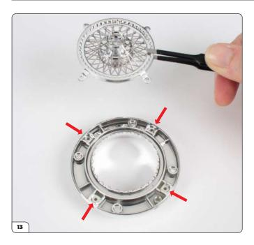
Fit the four tabs on the retainer ring into the recesses on the inner wheel rim (39VB-B).
