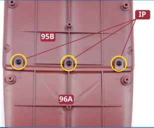
Take the keel section **95B** from the previous issue. Check how the three screw sockets at the aft end of **95B** connect with the screw holes in the tabs at the forward end of part **96A**. Fix them together with three **IP** screws.
