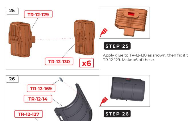
Glue TR-12-14 as shown and attach TR-12-169. Then attach the hinge TR-12-127.
