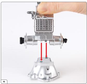
Take the gearbox assembly (stage 014) and align it with the bell housing.
