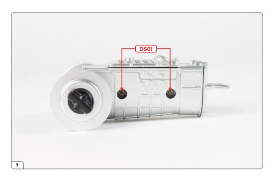
Fit the two parts together and secure with 2x DS01 screws.
