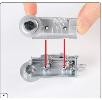
Align the left gearbox assembly (marked 'L') as shown.
