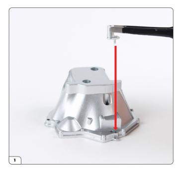
Take the bell housing (15-A) and align the clutch cylinder (15-B) as shown.
