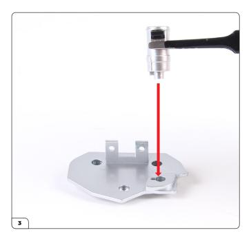
Align the starter motor with the bell housing cover (16-A), which has a shaped hole.
