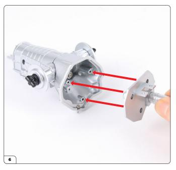
Align the bell housing cover with the gearbox assembly (stage 015).
