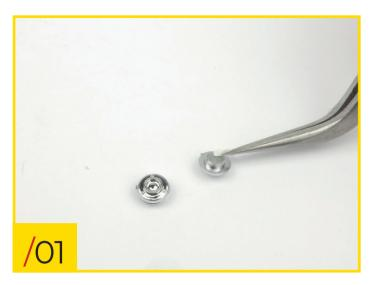
54/01 Remove the piece of protective paper from the underside of the two latch receivers.
