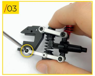
56/03 Connect the lower arm A (which has a central hole) to the rest of the assembly, orientating the pieces as shown. The longer end of the arm needs to be fitted to the mount; the shorter end goes to the stub axle. Screw a type B screw into the hole indicated.
