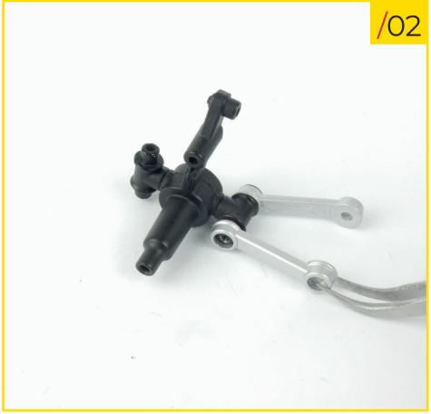
55/02 Fit the second upper arm to the stub axle, being very careful to ensure you orientate the pieces as shown in the photo.
