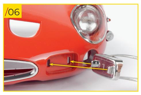
50/06 Now fit the left fog light into its position on the front of the body, as shown.
