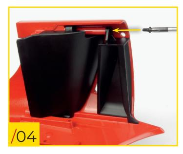
52/04 Fit the left secondary duct to the body and secure the pieces together with another type C screw.
