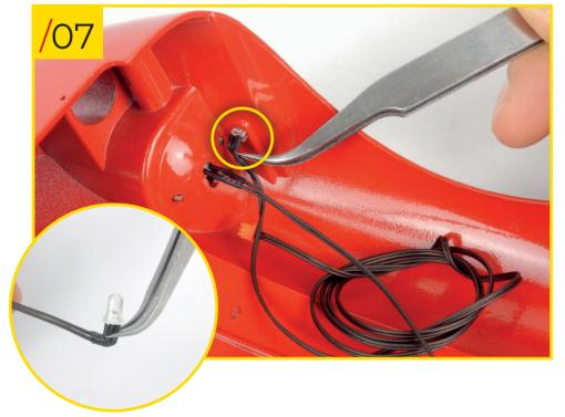
49/07 Working from inside the body, and making sure the sets of wires correspond to the correct side, insert the LED lights into the holes. Using a pair of tweezers to ensure you don't damage the components, bend the lights as shown in the round photo. Do not force them into the holes, you can use a small drop of PVA glue if necessary.
