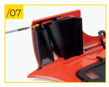
52/07 Finally, fit the right secondary duct to the body and secure it using another type C screw.
