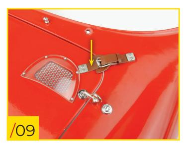
53/09 Stick the strap to the bonnet. When the model is finished, the bonnet can be opened by releasing the strap from the buckle and rotating the latch.
