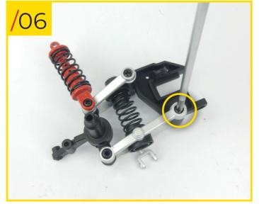
56/06 Working on the other side of the assembly, fit the lower arm B (the one without a central hole). Ensure that the longer end of the arm goes towards the mount, and the shorter end towards the stub axle, then insert the stud on the centre of the arm into the other side hole in the spring support. Screw a type B screw into the hole indicated by a circle in the photo.
