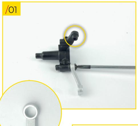
55/01 Fit one of the upper arms to the stub axle, orientating the pieces as shown. Use the stud highlighted by the circle in the photo as a reference for the orientation of the stub axle. The holes at the ends of the arms aren't identical: for this step you'll need to use the end with the larger hole (shown in the round photo). Secure the pieces together using a type J screw.
