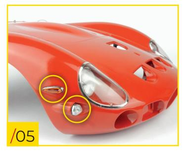
49/05 Repeat these steps to fit the second sidelight and the components for the right indicator, which are contained in a small bag marked "R".
