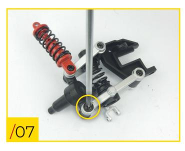
56/07 Screw a type J screw into the hole indicated to secure the arm to the stub axle.
