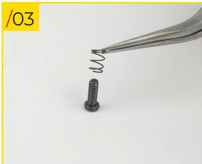
54/03 Slide the spring onto one of the type I screws.
