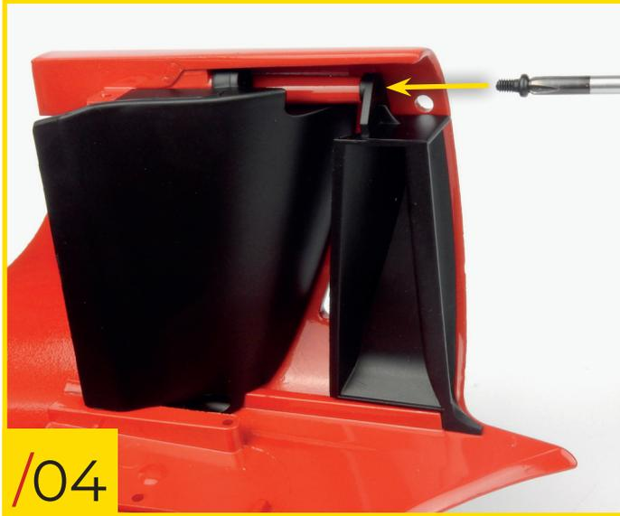
52/04 Fit the left secondary duct to the body and secure the pieces together with another type C screw.
