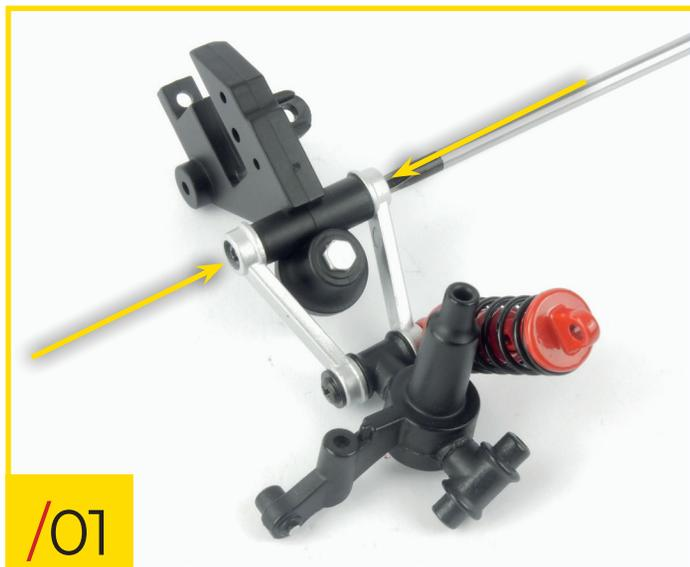
56/01 Place the suspension assembly you worked on in stage 55 and the connecting mount on your work surface. Orientate the pieces as shown and secure them together by screwing two type B screws into the holes indicated.
