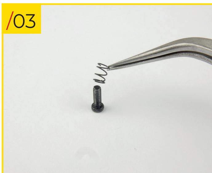
53/03 Now slide the spring onto one of the type I screws.
