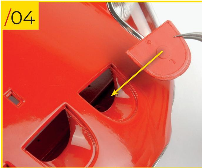
51/04 Now remove the backing from the lower cover with an "L" on it and fit it to the body, as shown.
