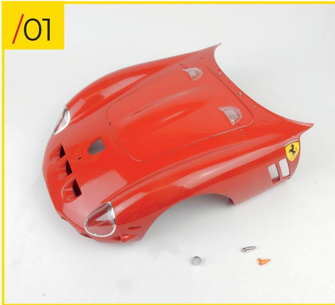
49/01 Place the front section of the body, one of the sidelights, the left indicator housing and the left indicator lens on your work surface. The housing and lens are inside a small bag with the letter "L" marked on it.
