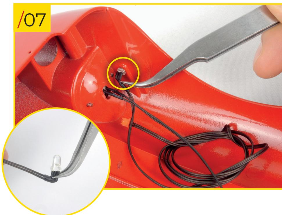
49/07 Working from inside the body, and making sure the sets of wires correspond to the correct side, insert the LED lights into the holes. Using a pair of tweezers to ensure you don't damage the components, bend the lights as shown in the round photo. Do not force them into the holes, you can use a small drop of PVA glue if necessary.
