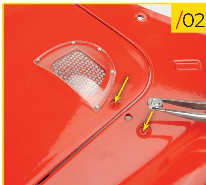
53/02 Working on the left side of the body's front section, insert the two receivers into their slots on the body and bonnet, orientating the pieces as shown. You can use a drop of PVA glue if necessary.
