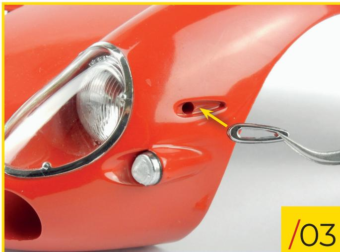
49/03 Fit the indicator housing into position, as shown in the photo...
