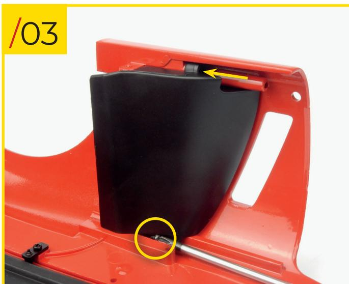
52/03 Secure the pieces together using two type C screws.
