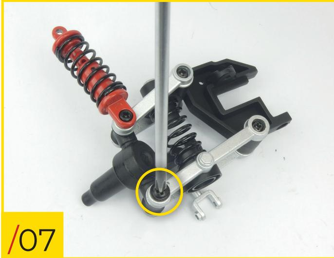
56/07 Screw a type J screw into the hole indicated to secure the arm to the stub axle.
