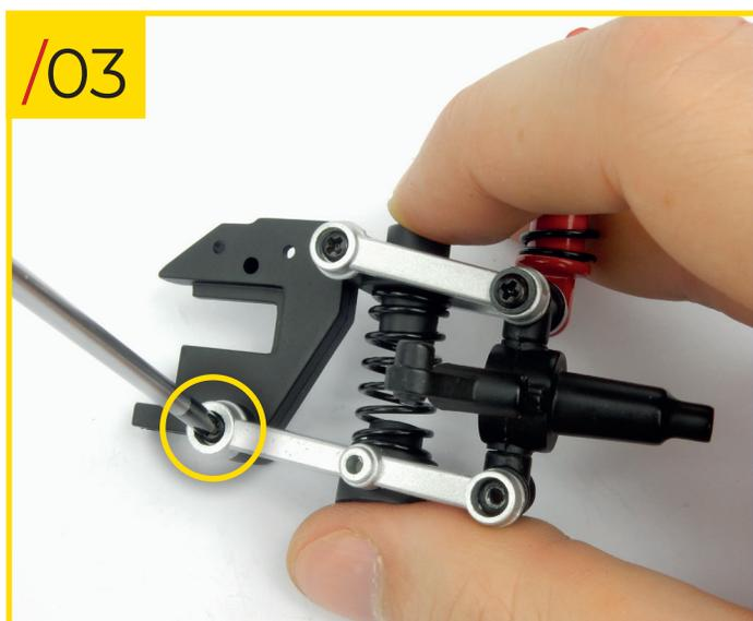
56/03 Connect the lower arm A (which has a central hole) to the rest of the assembly, orientating the pieces as shown. The longer end of the arm needs to be fitted to the mount; the shorter end goes to the stub axle. Screw a type B screw into the hole indicated.
