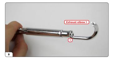
The flats with the number on (see picture 4) should face each other for correct alignment. Once all four pipes are firmly in place, hold the ends together and align the four ends with the exhaust plate. This is also engraved with the numbers 1–4 to assist with correct alignment.
