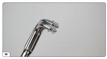
Note the correct orientation of the exhaust plate – the raised corners should face outwards towards the pipes (picture 10).
