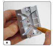
Then add the carburetor top, aligning the tiny hole with the corresponding lug (picture 3) in the corners, fixing the parts together using 2 x TYPE OP05 screws.
