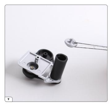
Align the end cap over the end of the dynamo, noting the projecting tab to ensure it fits the correct the way round.
