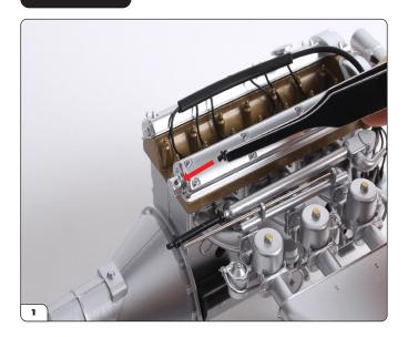
FIT THE REV COUNTER GENERATOR CONNECTOR TO THE EXHAUST CAM COVER
