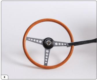
Press firmly into place, checking that the logo is correctly centred as shown
