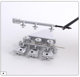
Align the three lugs on the air balance pipe with the three holes on the manifold and fit into position.
