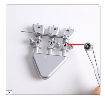
Take one of the suction chambers from the previous stage and press it into the key-shaped hole on the carburettor.
