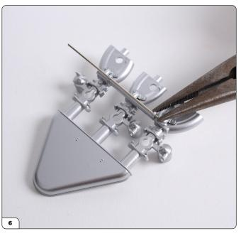
Using pliers, squeeze the ridged end of the shaft through the first small hole to anchor the shaft into position.
