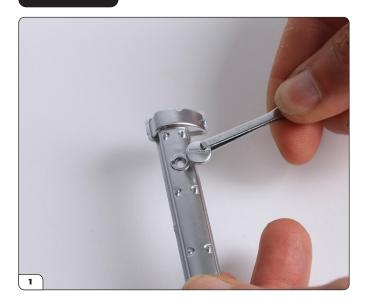
ASSEMBLE THE EXHAUST CAM COVER
