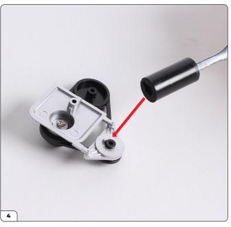
Align the keyhole-shaped hole on the end of the dynamo with the matching lug on the timing chain cover.
