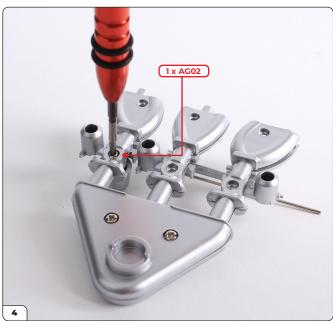
Fix in place from the reverse side using an AG02 screw.
