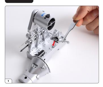
FIT THE FILTER HEAD AND HOSE TO THE ENGINE BLOCK ASSEMBLY FROM STAGE 04.
