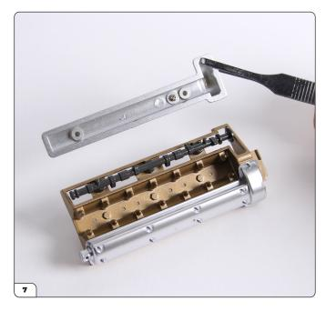
FIX THE EXHAUST CAM COVER TO THE CYLINDER HFAD
