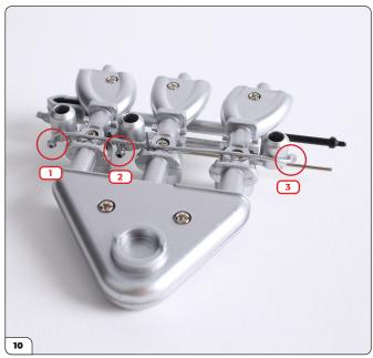
Using tweezers, push the hole on the left hand side of the pipe over the projecting pin on the lower float bowl (1). Connect the central hole on the pipe to the pin on the central float bowl (2), and then connect the remaining union to the pin on the third float bowl at the right hand side (3). Apply a drop of superglue if necessary.
