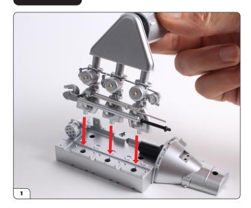
ATTACH THE CARBURETTOR ASSEMBLY TO THE ENGINE BLOCK
