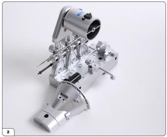
Press the filter head into position, allowing the pipe to project outwards from the block.
