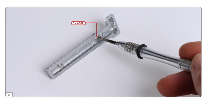
Secure in place from the reverse side using an AG02 screw.
