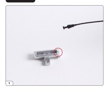
ASSEMBLE THE IGNITION COIL BEFORE FIXING IT TO THE CYLINDER HEAD, ALONG WITH THE ENGINE BREATHER.
