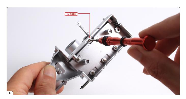
Secure from the reverse side using an AG03 screw.
