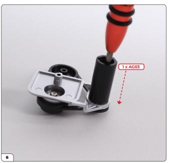
Fit an AG03 screw through the body of the dynamo and tighten to secure the dynamo in place.
