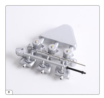
This shows the air balance pipe correctly positioned.
