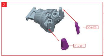
Glue rocker box parts 004-05 & 004-06 to the cylinders assembled in 1. Please note that 004-05 & 004-06 are different shapes. Ensure the holes face outward. Make two of these.
