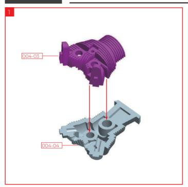
Apply a small amount of superglue to the two pins on part 004-03 and insert them into the holes on part 004-04 to join them. Make two of these.
