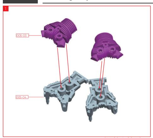
Apply a small amount of superglue to the two pins on part 005-03 and insert them into the holes on part 005-04 to join them. Make two of these.
