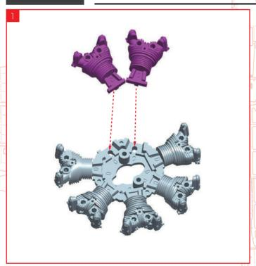
Insert the protrusions on the cylinders from STEP 1 into the holes marked C on the crankcase assembled in Stage 03. Do not glue.
