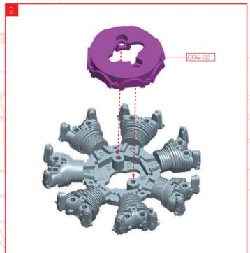
Cover the parts assembled in 1 with part 004-02.
