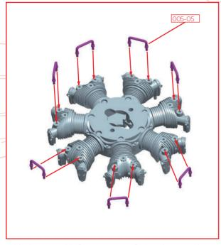
With the assembly from Stage 04 facing downwards, glue the oil pipes 005-02 to each of the seven cylinders.
