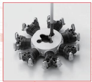
Fix the cover in place with  $2 \times 004-08$  screws. This is a temporary fastening, so don't overtighten it.
