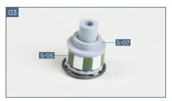
Push the green capstan drum **5-05** down the shaft as far as it will go. Then fit the capstan support **5-07** onto the shaft in the same way, pushing it down as far as possible.
