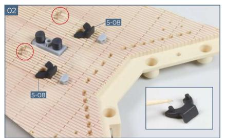
Place the first chain guide **5-08** on the work surface and apply a drop of superglue on the two small pegs on the underside (see inset). Fix in place on the upper deck. Repeat the process with the second chain guide **5-08**. The main image shows the two guides fixed in place.
