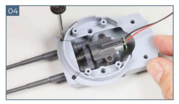
Fit the base plate on the housing and secure it with the six **PB** screws, as shown. A spare **PB** screw is supplied. Save it in a labelled container in case you need it later.
