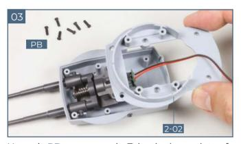
Have six **PB** screws ready. Take the base plate of the turret **2-02** and locate it on the turret housing, bringing the motor cable through the large opening, as shown.
