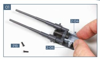
Fit the upper part of the motor mounting **2-04** on the cradle base plate **2-06**. A stud on the base of the motor mounting fits in a slot in the base plate.
