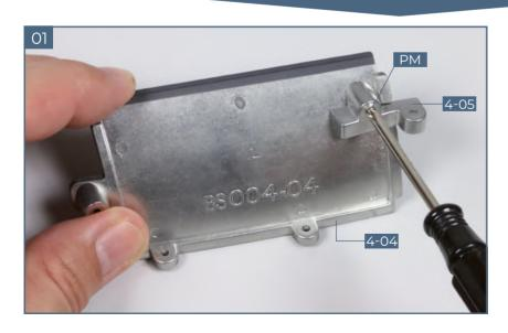
Take the connector **4-05** and position it on the hull section **4-04** as shown. Fix in place with a **PM** screw and put aside safely with the bow hull sections.
