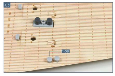
Glue the first two bollards **1-08** firmly into position in the large circular openings on the starboard (right) edge of the upper deck.
