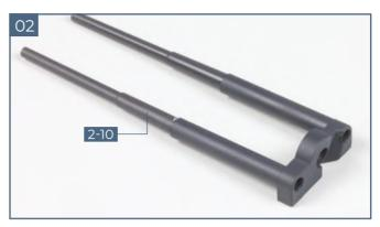
Repeat this process with the second barrel **2-10**. When gluing the two barrels, make sure that they are exactly aligned, so they are parallel, following the line of the barrel connector.
