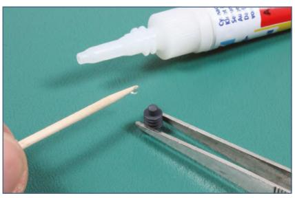
■ Always apply the superglue extremely sparingly! We recommend that you use superglue gel, which can be applied with pinpoint accuracy to the relevant surface using a toothpick.
