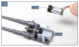
With the gun barrels pushed forwards, fit the motor **2-12** into the top of the motor mounting **2-04**. Make sure the motor is the right way round with the cables at the upper edge of the green board.
