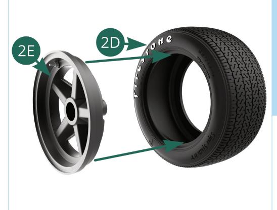
Firmly press the front wheel outer rim (2E) into the front wheel tyre (2D).
