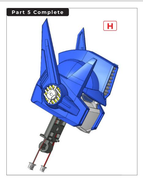
In the next steps, you will assemble the headlights and the chest. Before you begin, please test the LEDs are working correctly. Plug the battery box (TR-1-29) into the circuit board (TR-1-28), then plug the LEDs, one at a time, into the smallest plug on the circuit board. When plugged in, all four LEDs should light up.
