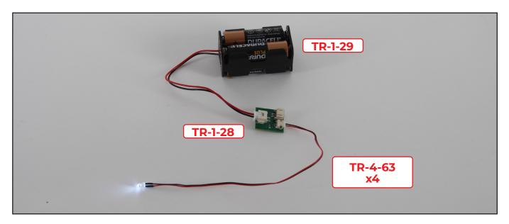
Note: Once the LEDs are assembled in the chest, they will be glued in place. It will be diffuclt to replace a faulty or broken LED if they are tested after assembly.
