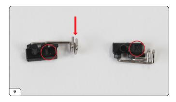
Next take a left and a right fuel injection nozzle (these are marked with "L" and "R" to distinguish them, shown circled above). Note that the left nozzles also have a slightly longer metal section (arrow).
