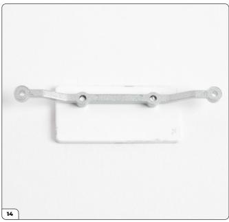
Press the bracket into place by fitting the holes of the bracket over the pins of the license plate.
