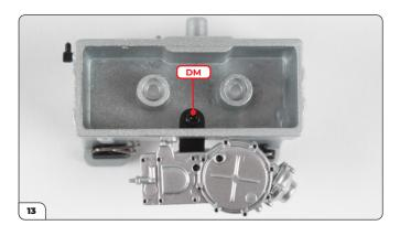
Fit the fuel meter into the housing and secure it using a DM screw.
