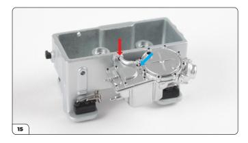
Starting with the straight end of the pipe, push it into the hole of the housing (red arrow), then fit the curved end of the pipe into the hole of the fuel meter cover (blue arrow).
