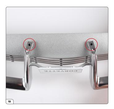
Turn the assembly over and align the tabs of the bumpers over the screw holes of the panel (circled).
