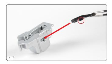
Take the fuel meter body and the bracket. There is a shaped slot in the body for fitting the bracket (arrow). Note that the bracket has a protruding notch (circled) to ensure it fits into the shaped slot in the correct orientation.
