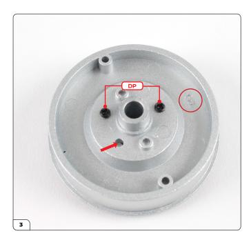
Turn the assembly over and lay it on your work surface as shown, noting the orientation of the '3' (circled). Secure the parts together using 2x DP screws in the indicated holes. Check you have identified the correct screw holes - one of them (indicated by an arrow) should remain free.
