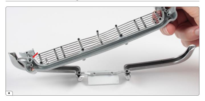
Start to fit the body panel into the bumpers by positioning the middle hole, highlighted in the previous step, under the bumper bracket (arrow). Once in place, carefully lower the panel into position on the bumpers.
