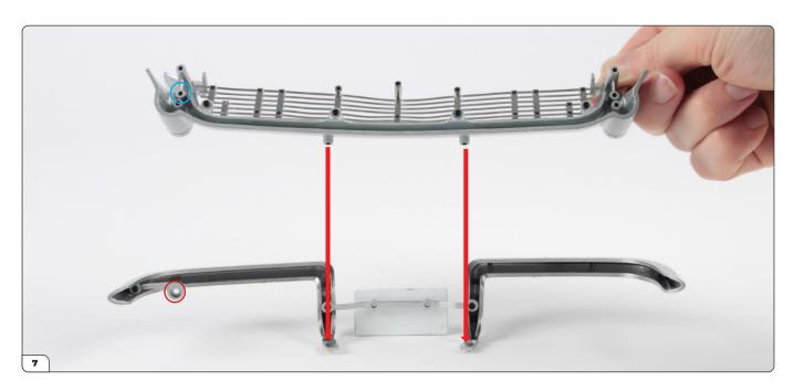
Retrieve the front body panel assembly from Stage 01 and align it with the bumpers as shown. There are two raised screw holes on the underside of the panel which fit over the tabs protruding from the bumpers (arrows). The bracket (circled in red) fits into the middle hole on the left-hand side of the panel (circled in blue).
