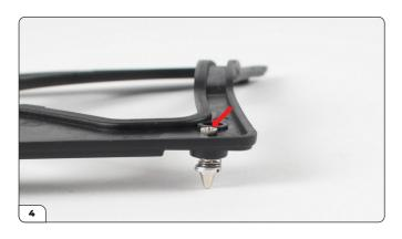
Push the narrow end of one of the latches through one of the holes, then secure it from the opposite side by twisting a hex nut over the threaded narrow end. Keep twisting until the tip of the narrow end is flush with the nut (arrow). Take care when securing the latch pins as you'll need to compress the spring at the same time.
