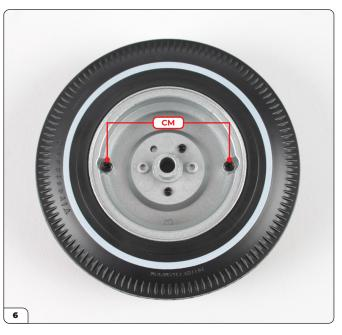
Fit the inner rim into the tyre then secure it using 2x CM screws. Check that the inner edge of the tyre is tucked neatly under the lip of the wheel rim
