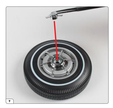
Turn the wheel back over and take the three-bar spinner. This pushfits into the recess of the wheel cover.
