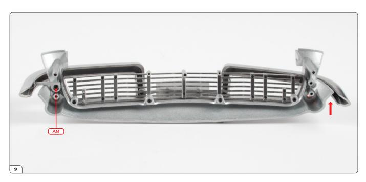
The assembly should look like this once the panel and bumpers are fitted together. Secure the bumper bracket and panel using an AM screw. Note that the right bumper and the right-hand side of the panel (arrow) will be loose for now, take care not to damage any parts while driving the screw in place.
