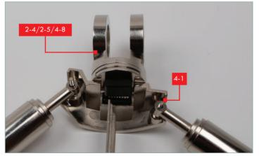
STEP 15 Insert the assembly 2-4/2-5/4-8 into the slot in part 4-1, as shown.
