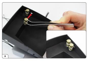
Push the blue peg on Fuel Pump Pipe 1 into the upper hole on Fuel Pump 1.
