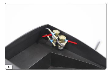
Push the blue peg on Fuel Pump Pipe 4 into the lower side hole on Fuel Pump 2. Push the free end of Pipe 4 into the end of Fuel Pump Pipe 2.
