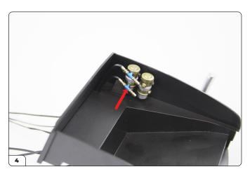
Push the blue peg on Fuel Pump Pipe 3 into the upper side hole on Fuel Pump 2. Push the free end of Pipe 3 into the end of Fuel Pump Pipe 1. Note: Pipe 3 has a 1 engraved on it, and pipe 4 has a 2 engraved on it.
