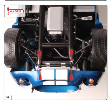
Take the Sway Bar Mounting brackets (100e) and fit them over the Anti-sway Bar. Secure each one using a TYPE OP17 screw.
