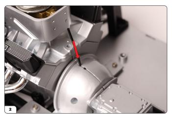
Take cable No. 07 from Stage 95 and thread it through the engine section, from front to back as shown. Leave equal lengths of cable projecting from both sides of the engine. Repeat on the opposite side with cable No. 08.
