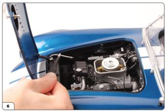
Take the Carburetor Actuator System (100c) and push the pins onto the the Steering Shaft Top Cover Plate (99d, pictures 8 & 9 below).
