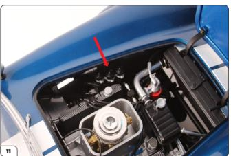
Locate the three pipes that have just been fed through from the Canister Set and attach them to the Mounting Box (stage 48).
