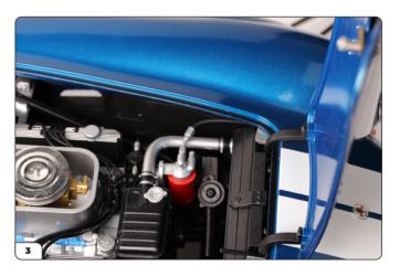
Take the Oil Vapour Canister Large Pipe (100b). Push one end into the Oil Vapour Canister (stage 66) and the other end into the Engine Block (see also picture 5 on the next page).
