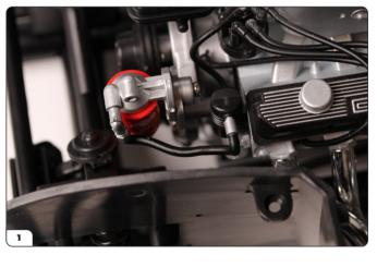
Take Pipe 99c and place one end in the hole on the Flywheel Cover as shown. The top end of pipe 99c is left unconnected for now.
