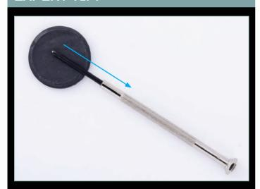
It is easier to position the screws if you have a magnetic screwdriver to pick up the screws. If your screwdriver is not magnetic, draw it across a magnet in one direction, as indicated by the arrow, to induce magnetism.
