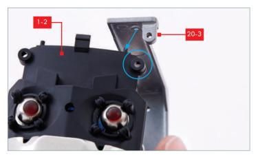
The tab with a screw socket at the front of the bracket **20-3** will fit in front of the screw socket at the top of the head (circled). There is a locating hole in part **20-3** which matches a locating peg on part **1-2**, shown above by the blue arrow.
