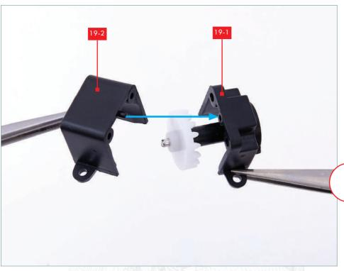
Take the cog assembly 19-1 and the housing 19-2. Check the fit of the assembly in the housing. The pin on one edge of the housing should be located in the socket on the cog assembly, as indicated by the arrow.
