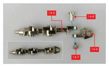
In the usual way, join part **14-6** to the finger assembly using connector parts **14-7** and **14-8**. The inset shows how the completed finger should look.
