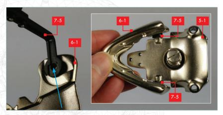
There are grooves on either inner side of part 7-5 (see above left) into which the screw sockets on part 5-1 slide. Part 5-1 is fitted from below as shown above, right.
