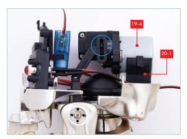
Fit the barrel of the motor 19-4 into the motor support, with the peg on the motor housing 19-1 through the loop.
