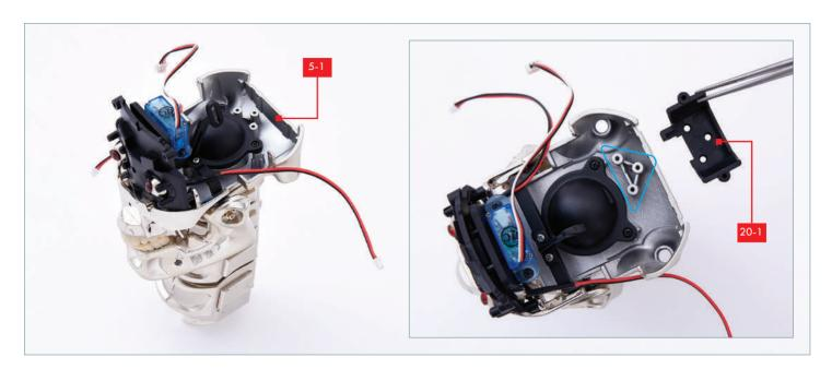
Take the head assembly from stage 18. Identify the three screw sockets (outlined) at the back of the head on part 5-1 (see inset). Align the screw sockets in the base of the motor support 20-1 with the screw sockets on part 5-1.
