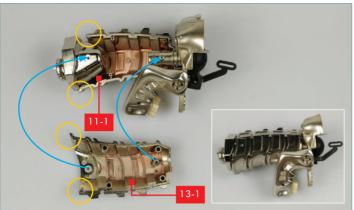
Turn the assembly over and take neck part 13-1; note the small holes, circled in yellow. These holes receive small pins, also circled in yellow, on part 11-1. Test-fit part 13-1 on top of part 11-1 as shown in the inset, aligning the holes marked by blue arrows.
