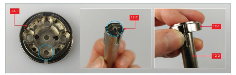
Again, taking note of the position of the screw holes and grooves in part 12-1 and 12-2, place the parts together.
