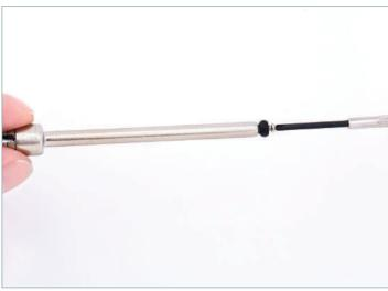
Take a lower arm B 16-3, a rubber washer 16-4 and a screw PB 2x6 mm (16-6). Fit the washer over the screw and then fix the screw into the narrow end of part 16-3.
