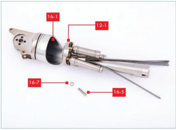
You will now need the arm and muscle assembly from stage 14. Note that there is a recess in the parts from stage 14 and a raised tab on the inside of part 16-1 (circled).
