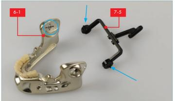
Now, take the lower jaw (6-1) from stage 06 and the head motor joint (7-5) from stage 07 and note the locating pins (marked with blue arrows) on part **7-5**. Note also, the matching holes (circled in blue) in the jaw part (6-1).
