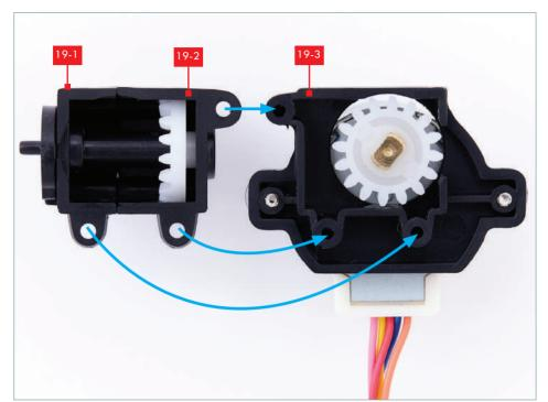
Check the fixing points on the cog assembly and housing 19-1 and 19-2 and the motor housing 19-3, as indicated by the arrows.
