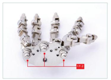
Fit the three ball joints 17-2 into the recesses in the palm of the hand.
