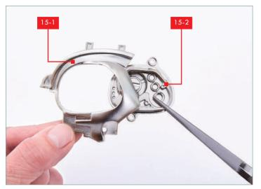
Take the two parts of the left head, 15-1 and 15-2. Fit the inner part 15-2 into the opening in part 15-1, as shown.
