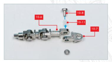
Position the next finger section 10-7 next to part 10-6. Fit connector 10-8 and sleeve 10-11 into the holes in parts 10-6 and 10-7. Note that the direction in which the connectors are inserted alternates.
