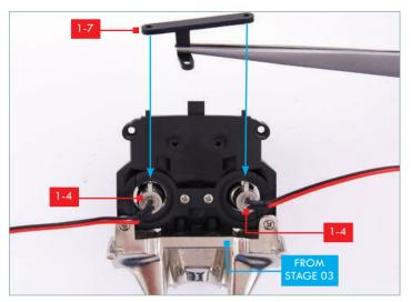
Take part 1-7, supplied with stage 01 and the head assembly from stage 03. Hold part 1-7 with the 'L' shape at the bottom, with the base of the 'L' pointing towards you. Fit the two holes in the top crossbar of part 1-7 over the two pins on parts 1-4, as indicated by the arrows.
