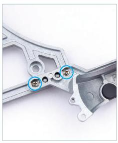
Carefully turn the assembly over, holding the nuts in place. Fix part **37-1** in place with two PM 2x6 mm screws (circled). The screws are held in place by the M2 nuts.
