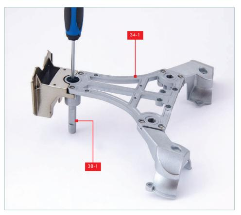
Turn the assembly over and fix the shaft **38-1** in place with a PM 3x6 mm screw.
