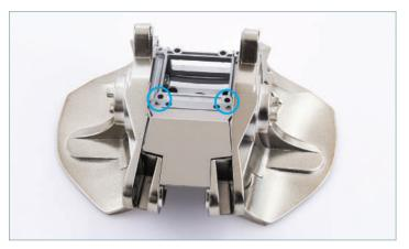
Turn the assembly over and identify the next two fixing points (circled).
