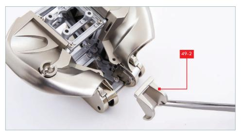
Take the pelvic plate **49-2** and position it in the orientation shown, so that you can fit it into the gap in the front of the pelvis.
