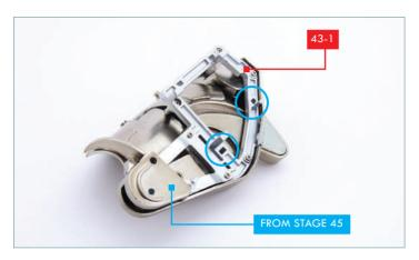
Take the assembly from stage 45. Identify two slots in the pelvic frame 43-1 (circled in blue) where the central frame will fit. The slot on the left is below a tab, and the one on the right is above a tab.
