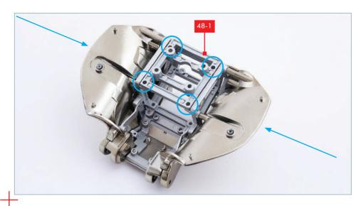
The tight fit of the tabs creates a fairly stable assembly, but ensure that the parts are pushed as close together as possible. The screw holes near the corners of part 48-1 (circled) should align with screw holes on tabs in the frames on either side.
