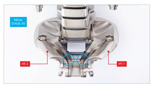
Take the assembly from stage 50 and identify the two holes in the pelvic shields **48-2** and **49-1** where the plate will fit (circled).
