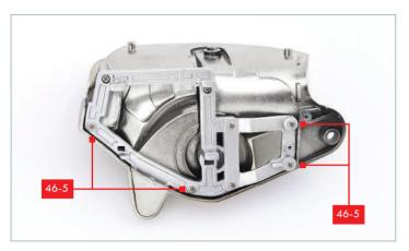
Use four PB 2x4 mm screws (**46-5**) to fix the pelvic frame in place, as shown here.
