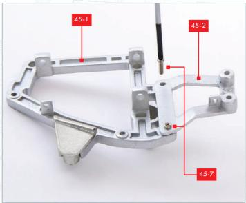
Turn the frame **45-1** over, ensuring that the nuts stay in place. Position part **45-2** so that the two screw holes align with the recesses in part **45-1**. Note that there are raised areas around the holes in part **45-2** (on the underside, when viewed from this angle), which fit into the recesses in part **45-1**.
