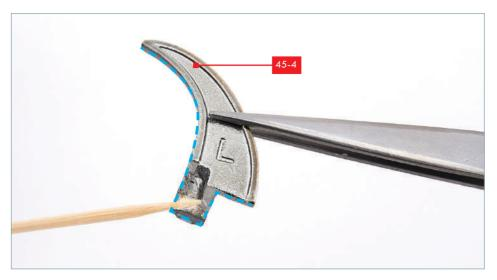
Apply a very small amount of superglue to the edges of part **45-4** that will be in contact with the assembly (highlighted with a blue dotted line).
