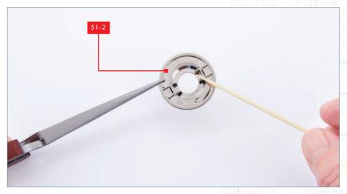
Apply a little superglue in the inner recesses of the hip socket **51-2**.
