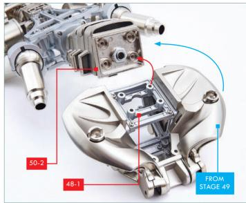
After checking the spinal cord **42-4** is still fully tightened, fix the connecting plate **50-2** in place by tightening the M10 nut **50-4** on to the end of the spinal cord, as shown. If necessary gently tighten with a suitable spanner or pair of pliers taking care not to over-tighten.
