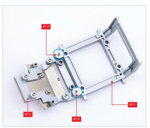
This shows the frame parts fixed together, with the PM 2x6 mm screws, circled.
