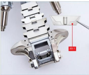
Take the pelvic plate **50-1** and identify the four raised pegs on the back of the plate, near the corners. Part **50-1** fits across the back of the pelvis at the base of the spine. The four pegs fit into the four holes (circled).
