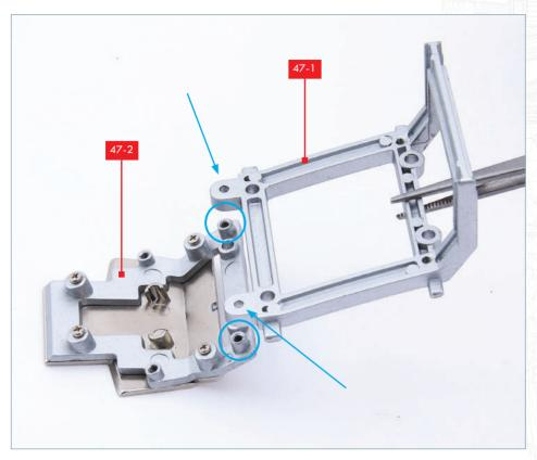
Take the rear part of the pelvic frame 47-1 and identify the two tabs with screw holes in them (arrows). Align the holes in the tabs with the raised screw sockets on part 47-2 (circled).
