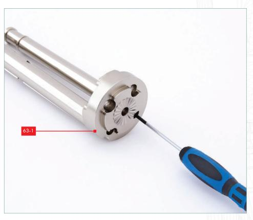
Fit the end of part 64-2 against the hole in part 63-1 (as shown in step 2). Fit the screw and housing into the corresponding hole on the other side of part 63-1 and fix in place. Note that **64-2** is not a tight fit against part 63-1; it hangs loosely.
