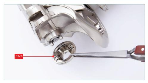
Fix the hip socket **53-2** in place on the side of the pelvis, so that the pegs on the pelvis go into the recesses in the hip socket.
