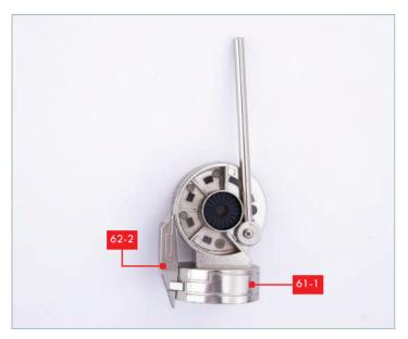
Fit the assembly 62-2/62-3 in place on part 61-1.
