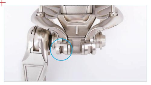
Take the assembly from stage 58 and identify the fixing point for the muscle near the centre of the pelvis (circled). Note that the model assembly is lying face upwards at this stage.
