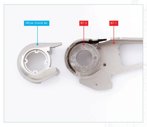
Fit all four M2 nuts in place then take the leg joint assembly from stage 86. Check how it fits over the end of the thigh 87-1.
