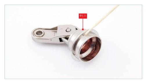
Take the muscle connector **91-1**. Apply a little glue around the side of the part, beneath the rim, as shown.
