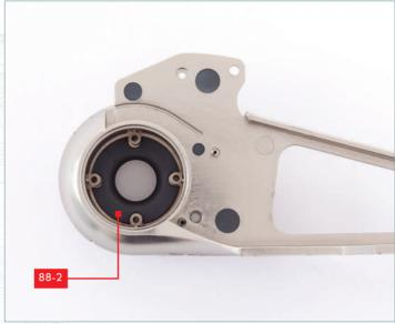
Take the thigh from stage 87 and place it in the orientation shown. Fit the inner hip joint casing 88-2 into the opening for the hip joint. The flat surface of part 88-2 is upwards, as shown.
