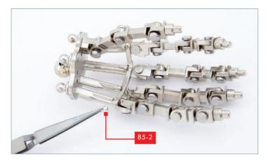
Fit the connector **85-2** into one of the rectangular sockets in the hand. Repeat to fit all four connectors in place.
