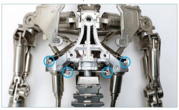
STEP 10 This shows the four screws in place (circled).
