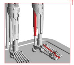
Connect the third toe and foot parts and add a second part to the lower leg.
