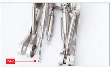
**STEP 10** Take the tendon **94-2** from this stage, with the **M3** nut. Fit the tendon assembly into the end of the muscle fitted in the previous steps.
