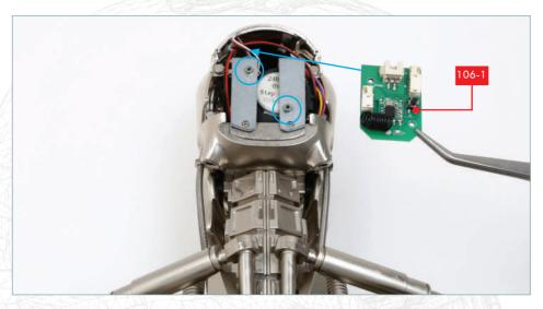
Position your model face down on the work surface. Position the circuit board 106-1 on the plates in the back of the head so that the two holes in the circuit board are aligned with the raised screw sockets (circled).
