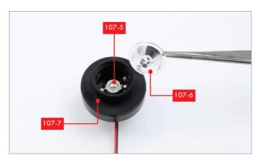
Turn the housing over and fit the lens 107-6 into the opening in the housing part 107-7, covering the LED 107-5. The flat side of the lens should face outwards. Push it in place until it clicks.
