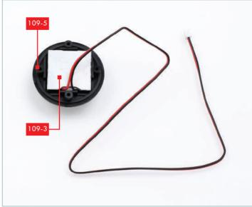
Take the LED 109-3 and bend the cables so that they fit through the recess in the edge of the circuit board and then bend away from the back of the circuit board.
