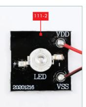
Check the two LEDs: part 111-1 has a red spot at the centre of the LED and a longer cable. LED part 111-2 has a plain clear centre. This will be important when you come to fit the searchlights.
