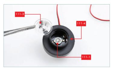
Turn the housing over and fit the lens 111-3 into the opening in the housing part 111-4, covering the LED 111-1. The flat side of the lens should face outwards. Push it in place until it clicks.
