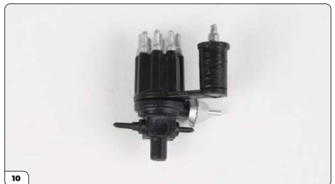
10 Fit the ignition coil onto the distributor.
