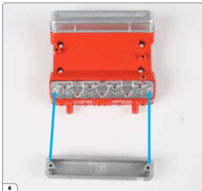
Align the right valve cover with the cylinder head (arrows).
