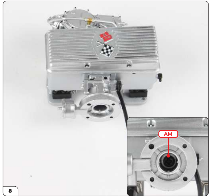
Push into place and secure with an AM screw (inset).
