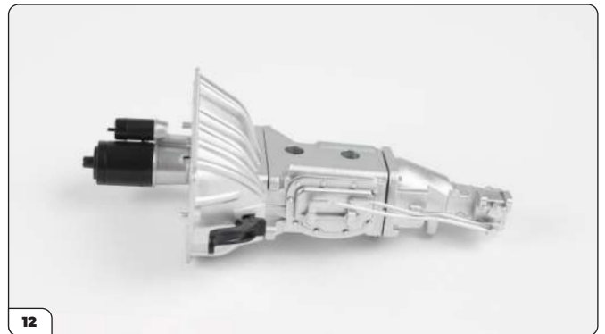
Push the starter coil onto the pin.
