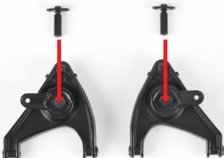
Turn the control arms over and fit the cylinders through the large holes (arrows).
