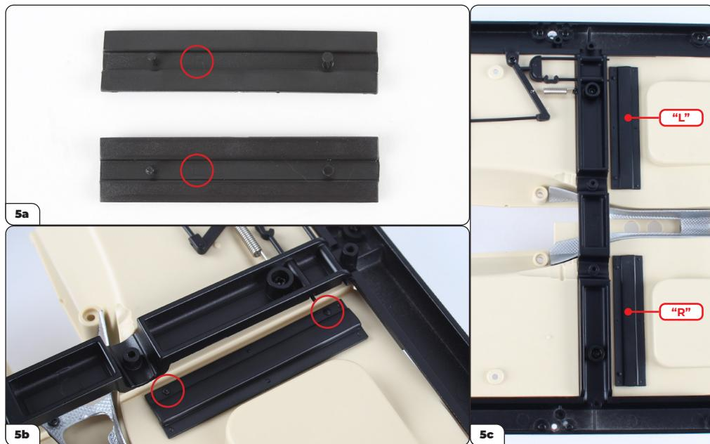
The chassis reinforcements are marked "L" and "R" to distinguish left from right (5a, circled). When fitting the chassis reinforcements, make sure the bolts are next to the frame's cross beam (5b, circled). Press the left and right reinforcements into position as shown (5c).
