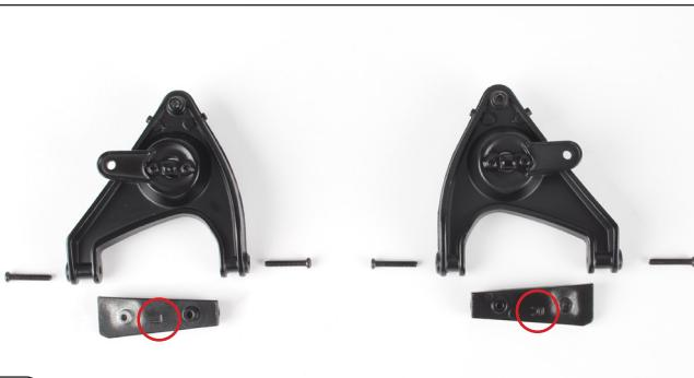
Align the shafts (marked "L" and "R", circled) with the control arms as shown, then prepare 4x KM screws which will secure the shafts from the outside of the arms.
