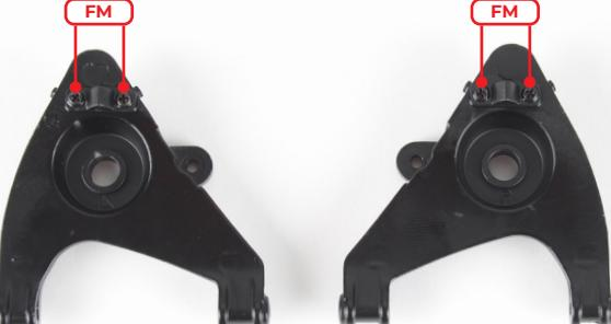
Place the brackets onto the control arms as shown then secure in place using 4x FM screws.
