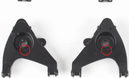
Lay out the lower control arms and the brackets. The control arms are marked with "L" and "R" to distinguish left from right (circled).
