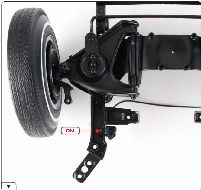
Fit the linkage bracket in the recess on the front chassis and secure using a DM screw.
