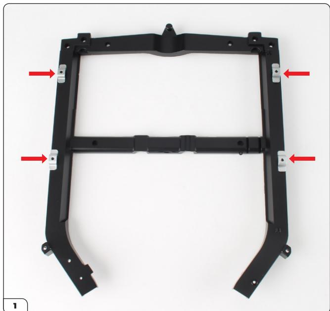
Position the mounting brackets on the chassis frame (arrows).
