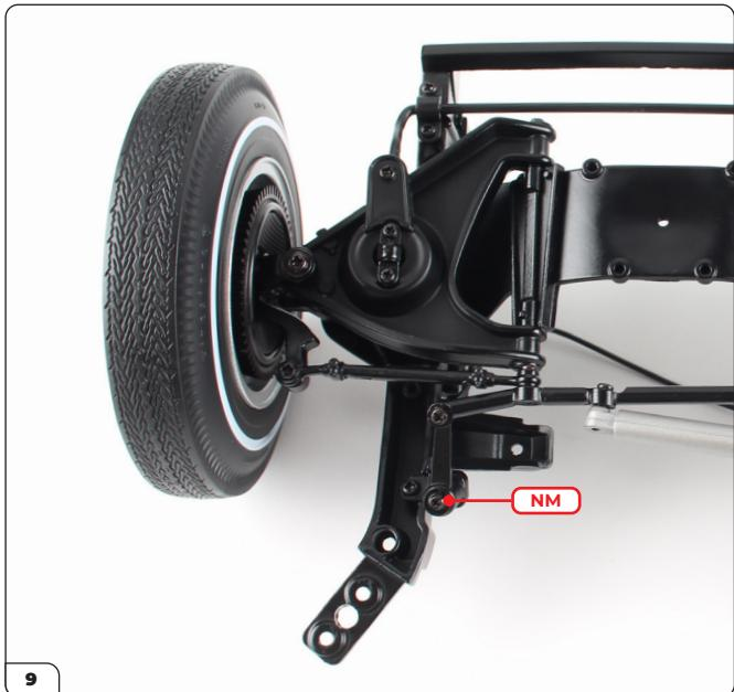
Secure the end of the idler arm to the bracket with an NM screw.
