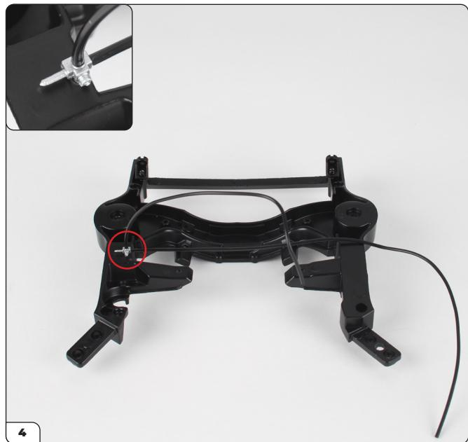
Press the bypass into the hole in the front chassis (circled).
