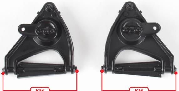
Fit the shafts in place then secure using the KM screws.
