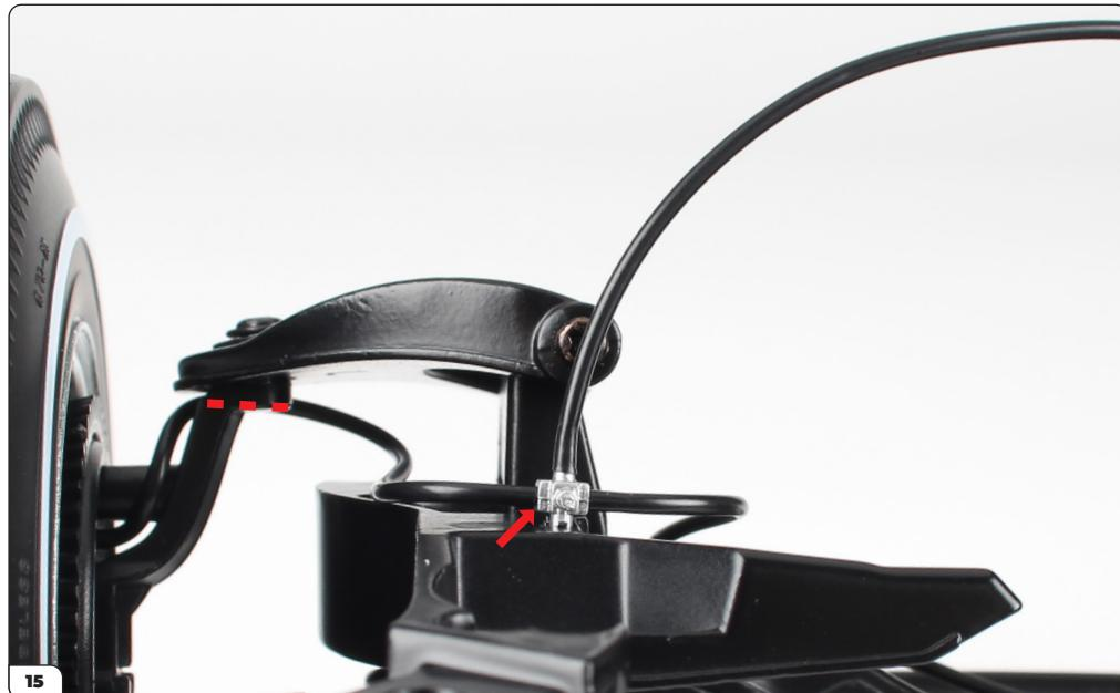
Take the loose end of the left wheel's brake hose and pass it behind the upright (dashed line) then feed it through to attach to the bypass (arrow) as shown.
