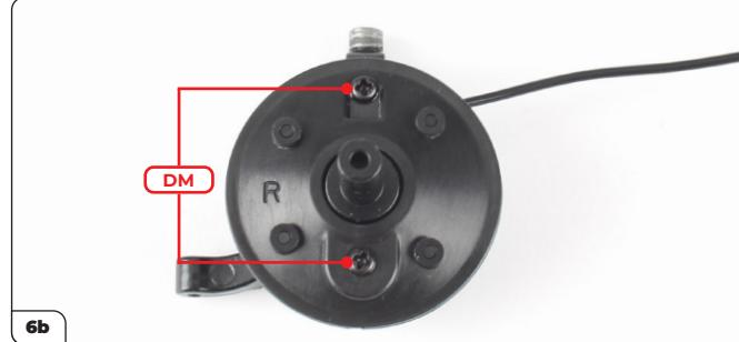
Fit the cover onto the right suspension upright as shown (6a) then secure using 2x DM screws (6b).
