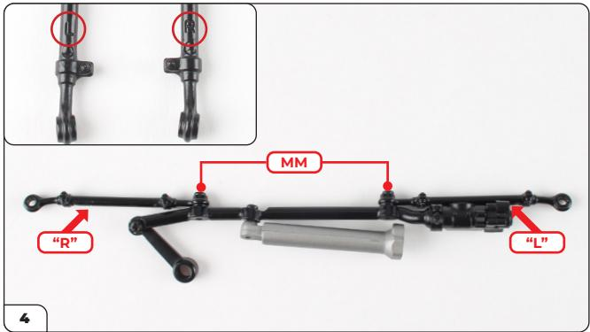
Fit the steering linkages (marked "L" and "R", inset, circled) and secure them to the steering bar using 2x MM screws. Note that the "L" and "R" marks should be located in the positions indicated by the arrows.
