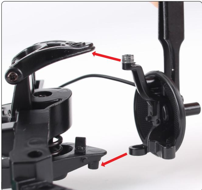
Align the upright with the chassis as shown. Fit the screw posts into their fixing points (arrows).
