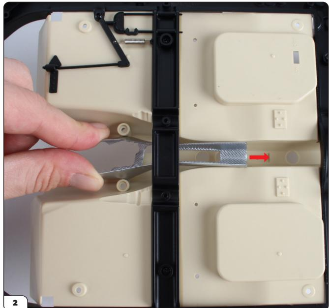
To fit the heat isolation shield, carefully squeeze the wide end and push it through underneath the cross beam, passing between the screw columns as shown.
