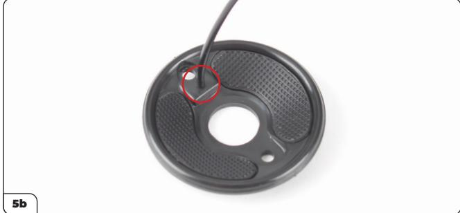
Remove the longer brake hose from the bypass (5a, arrow) then fit it onto the pin of the brake drum cover (5b, circled).
