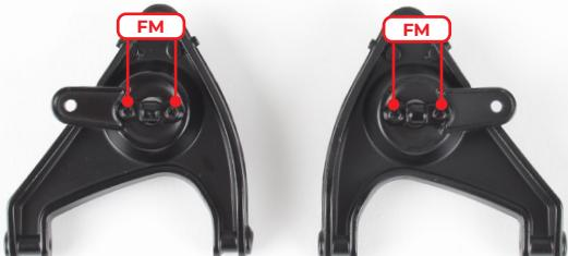
Secure the cylinders using 4x FM screws.
