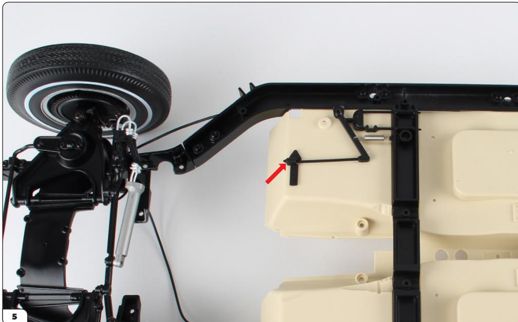
Fit the bushing over the handbrake cable (arrow) and press into the cockpit floor.
