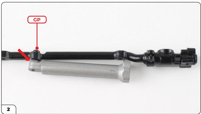
Position the cylinder onto the central steering bar as shown (note the rounded side of the cylinder is in contact with the bar, arrow) then secure using a GP screw.
