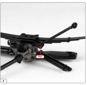
Secure using a PM screw.
