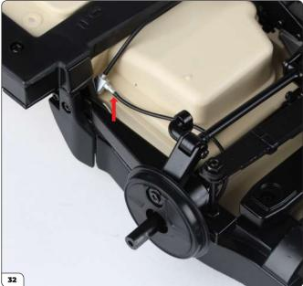
Plug the brake hose attached to the knuckle onto the pin of the silver connector (arrow).
