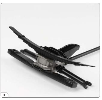
The leaf spring should curve upwards once in place.
