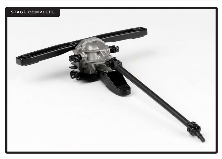
In this stage you'll fit the rear leaf spring suspension to the differential case. You'll also add the handbrake hoses to the main assembly.
