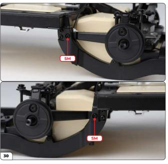
Check the upper control arms are aligned with the screw holes in the rear chassis side panels then secure each using an SM screw.
