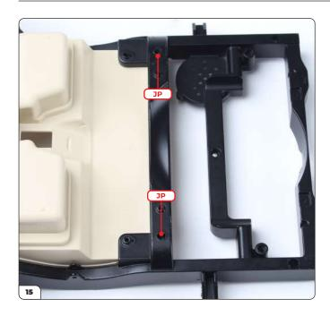
Drive  $2x\ JP$  screws through the holes in the rear chassis into the cockpit floor.
