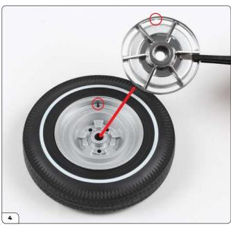
Turn the assembly back over and fit the six-spoke wheel cover in position, aligning the indent of the cover with the air valve (circled).
