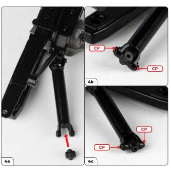
Fit a universal joint into the end of the axle drive shaft (4a, arrow) then secure using 2x CP screws (4b). Fit the other universal joint into the remaining axle and secure with 2x CP screws (4c).
