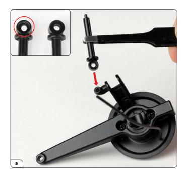
Position a rear damper rod over the lower control arm of the left knuckle (arrow). Note that the rod has a recess on one side (inset, circled) which should face out from the control arm.
