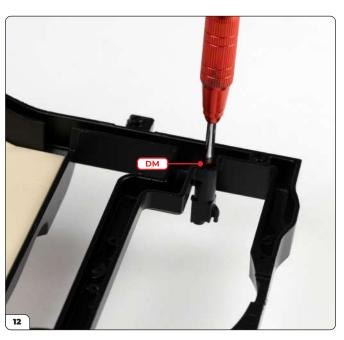
Flip the assembly and secure the bracket with a DM screw.
