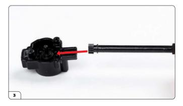
Place the transmission gear shaft into the gear box so that the end with teeth connects with the drive gear (arrow).
