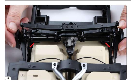
Press both damper rods into the cylinders (arrows), then fit the ends of the upper control arms into the openings highlighted in step 23.
