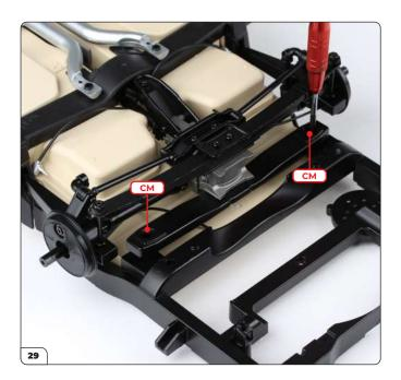
Secure the cross member to the rear chassis using  $2x\ CM$  screws.
