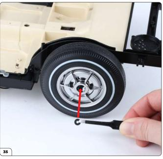
Fit the rear left wheel onto the knuckle as shown, then place a thin washer over the end of the post (arrow).
