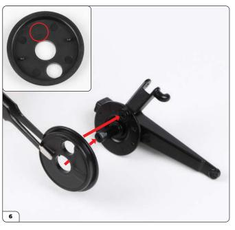
Place the left brake drum cover, marked with an 'L' (circled, inset), over the knuckle as shown.
