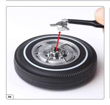
Remove the three-bar spinners from the wheels assembled in stages 25 and 27, if necessary.
