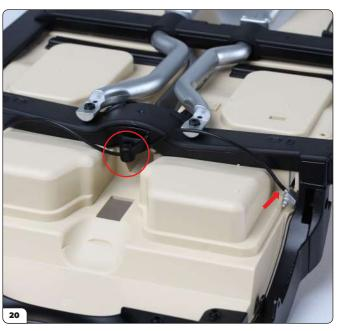
Run the cable under the protrusion of the chassis frame (circled) and plug the other end onto the top pin of the left-hand connector (arrow).
