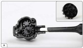
Fit the drive gear in place so that the side with eight teeth (inset) connects with the transmission gear.
