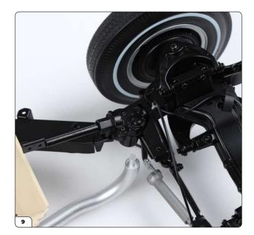
Place the gear box assembly into the recessed area as shown.
