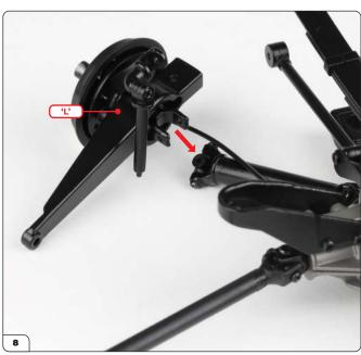
Align the left knuckle with the axle drive shaft on the differential's left side as shown (arrow).
