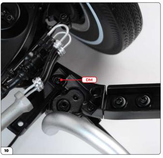
Carefully turn the assembly over and secure the gear box using a  $\ensuremath{\mathsf{DM}}$  screw.
