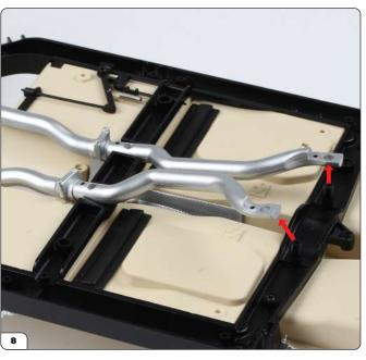
Gently lift the ends of the exhaust pipes from the chassis frame's screw posts (arrows).
