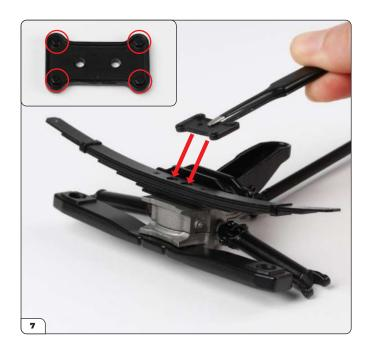
Place the leaf spring plate in position (arrows), ensuring the side with the bolts (inset, circled) is facing up.
