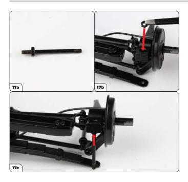
Fit the other strut rod to the right side in the same way. Screw a hex nut onto the long thread (17a), then place a hex nut in the hole of the upper control arm (17b). Screw the strut rod through from the other side (17c).
