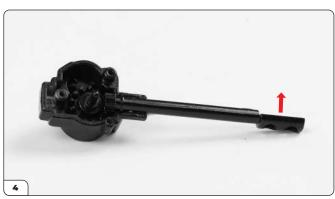
Twist the shaft so that the flat side of the other end is facing the direction shown by the arrow. The gears should turn when the shaft is twisted.
