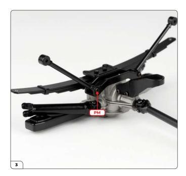
Fit the other lower swing bar and secure using a PM screw.
