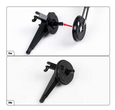
Place the right brake drum cover, marked with an 'R', over the knuckle.
