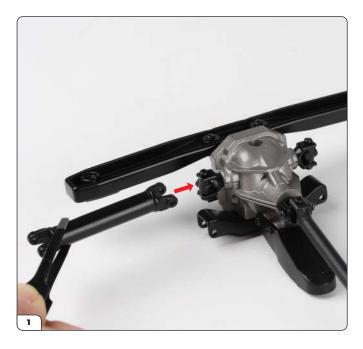
Position the end of an axle drive shaft onto the rear differential's joint as shown (arrow).
