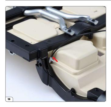
Plug one end of the long brake hose (130 mm) onto the top pin of the right-hand connector (arrow).
