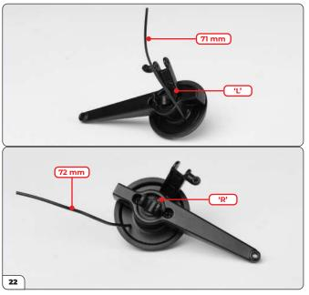
Plug the shortest brake hose (71 mm) onto the pin of the left knuckle and the slightly longer brake hose (72 mm) onto right knuckle.
