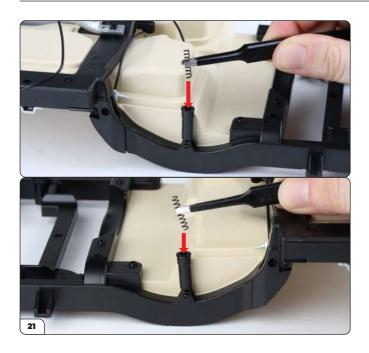
Place the two springs inside the cylinders as shown (arrows).
