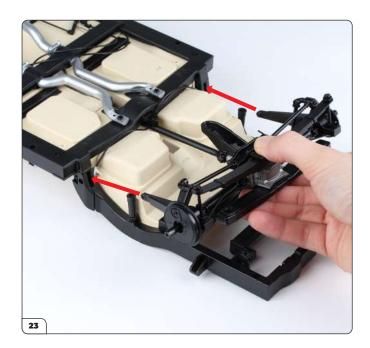
Continue to move the transmission shaft through the central channel, while guiding the upper control arms towards the openings of the rear chassis (arrows).
