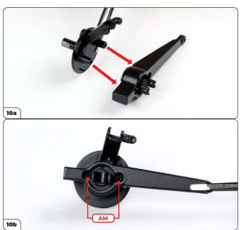
Fit the right knuckle into the upper control arm (10a) then secure using  $2x \, AM$  screws (10b).
