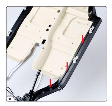
Use the pieces of adhesive tape to secure the main brake hose to the chassis (arrows).
