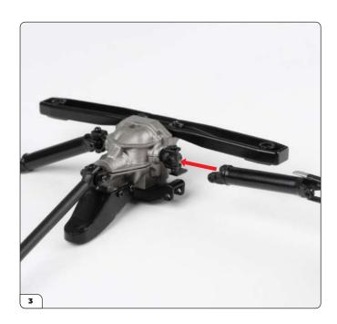
Fit the other axle on the remaining joint (arrow).
