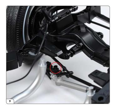
The round hole of the linkage fits onto the post of the central steering bar (circled).
