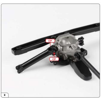
Secure using 2x CP screws.
