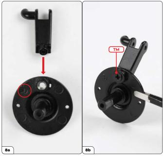
Fit the right lower control arm into the rear right knuckle, marked with an 'R' (8a, circled). Secure using a TM screw (8b).
