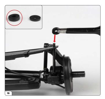
Place a thick washer (inset, circled) over the short rod end (arrow).
