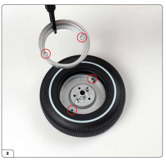
Turn over and fit the inner wheel rim onto the outer rim, aligning the holes (circled).
