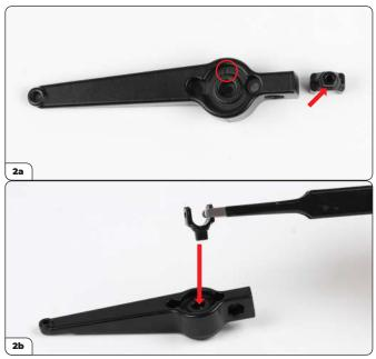
Take the left upper control arm (2a, marked with an 'L', circled) and a transmission shaft connector. Note it has a D-shaped post (2a, arrow). Fit the connector into the control arm (2b).
