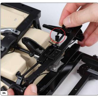
As you fit the assembly, guide the damper rods into the cylinders (circled).
