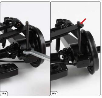
Flip the assembly and tighten the hex nut fitted in step 12 (using the spanner supplied) to secure the strut rod (14a). Fit the end of the leaf spring over the short threaded end of the rod (14b, arrow).
