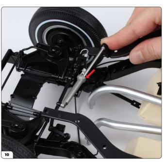
Push the cylinder bracket into the hole of the cylinder (arrow).
