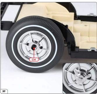
Fit the rear right wheel in the same way, placing a thin washer then securing it with a CM screw. Press the three-bar spinner in place (inset).
