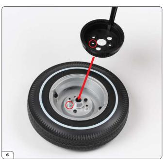
Fit the rear right brake drum onto the outer wheel rim using the locking pin and hole to align the parts correctly.
