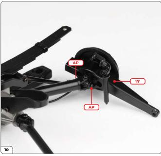
Fit the knuckle onto the axle and secure using 2x AP screws.
