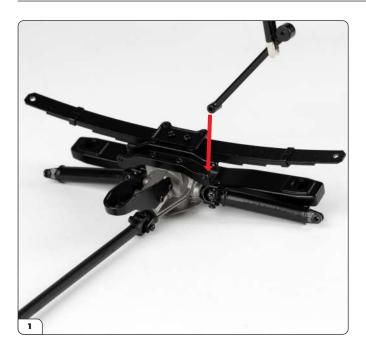
Fit the smaller end of a lower swing bar into the bracket of the rear differential (arrow).
